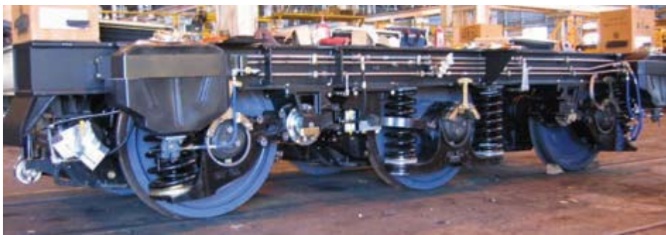
Figure 36: Semi-steering bogie as fitted to the SCT class locomotive [8]
