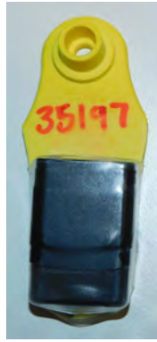
Figure 4.2 Axivity AX3 tri-axial accelerometer attached to a standard ear tag
