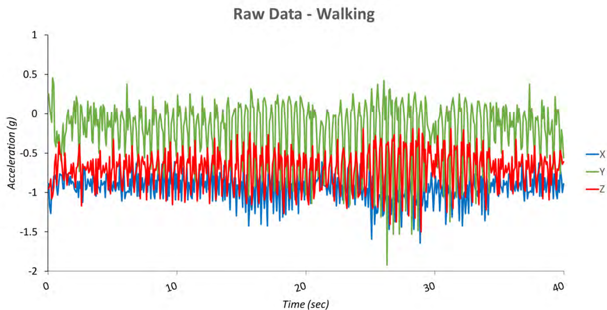
Figure 4.12 Acceleration signal from the ear-borne accelerometer while the animal was walking (40 s).
