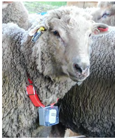
Figure 4.3 In-situ photograph of attached GNSS collar and accelerometer ear tag
