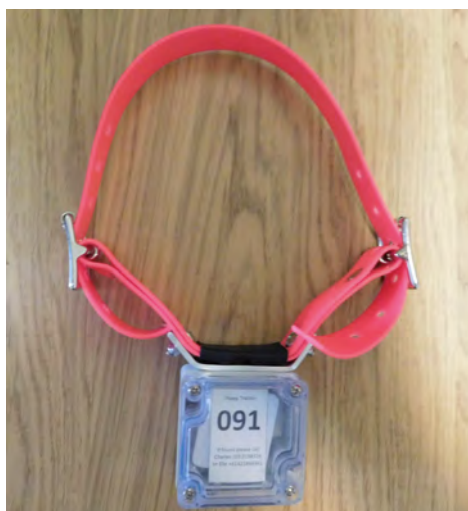
Figure 4.1 i-gotU GT-600 GNSS loggers enclosed in a neck collar
