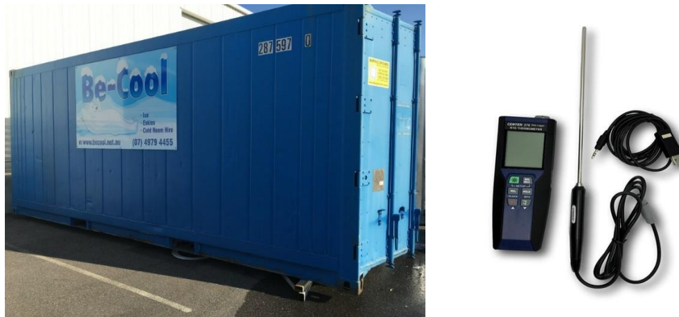
Figure 62. Right panel: Refrigerated container (20ft) capable of holding 24 tons of fruit. Left panel: insertion thermometer with data logger.
