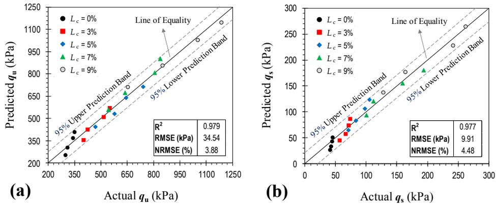
Fig. 1. Predicted versus actual data, along with the corresponding 95% prediction bands, for various soil-lime mix designs: (a)  $q_u$  (Eq. (15)); and (b)  $q_s$  (Eq. (16)).
