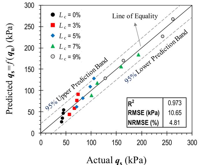
Fig. 3. Predicted (by Eq. (20)) versus actual  $q_s$  data, along with the corresponding 95% prediction bands, for various soil-lime mix designs.
