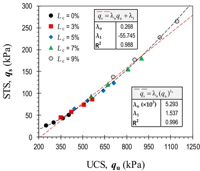
Fig. 2. Variations of  $q_s$  (predicted by Eq. (16)) against  $q_u$  (predicted by Eq. (15)) for the tested mix designs.
