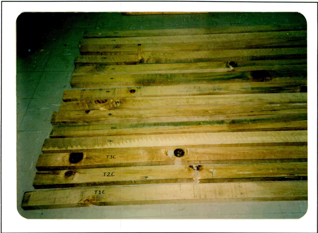
Photo 27: Tensile strength failures (t1c to t14c, treated), Aug 1993 (1694/3)
