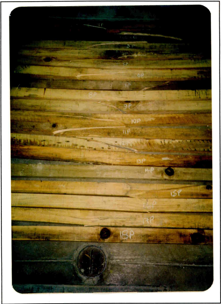
Photo 17: Bending strength tests (b1p to b18p, untreated) Feb 1993 (Y002/3)
