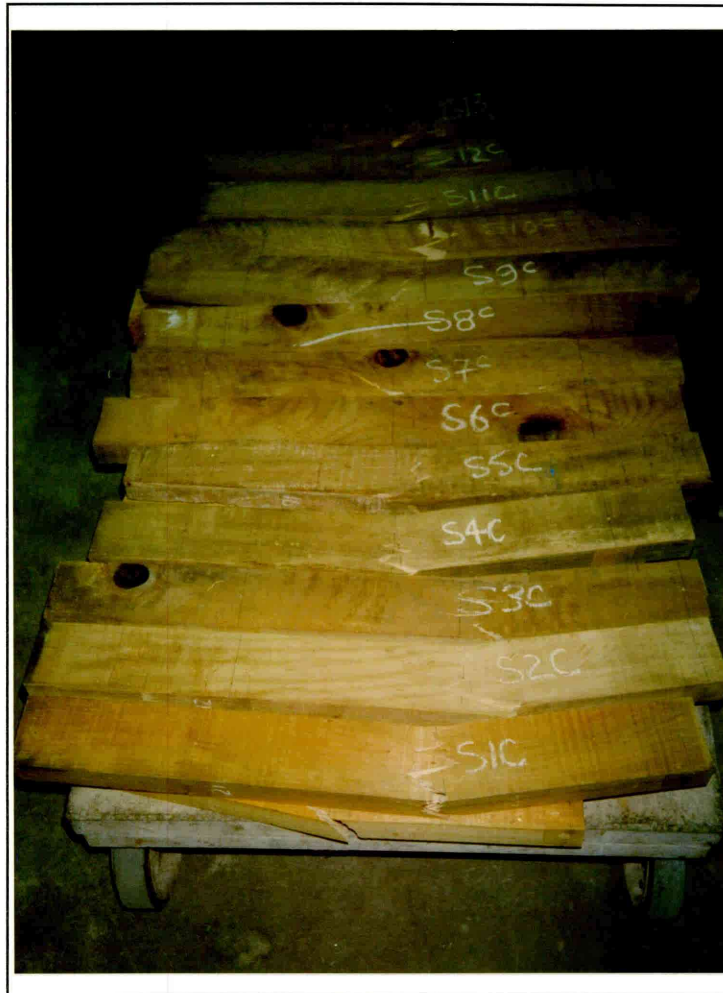
Photo 15 : Shear strength tests (s1c to s13c, treated) Feb 1993 (9934/1)
