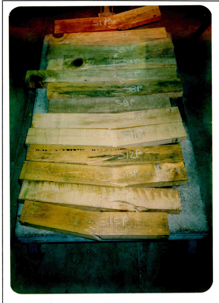
Photo 14 : Shear strength tests (s1p to s15p, untreated) Feb 1993 (9934/0)
