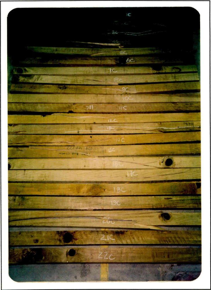
Photo 18 : Bending strength tests (b1c to b22c, treated) Feb 1993 (Y002/11)
