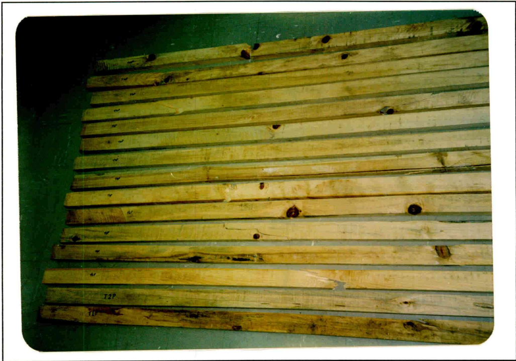
Photo 26: Tensile strength failures (t1p to t15p, untreated), Aug 1993 (1694/0)
