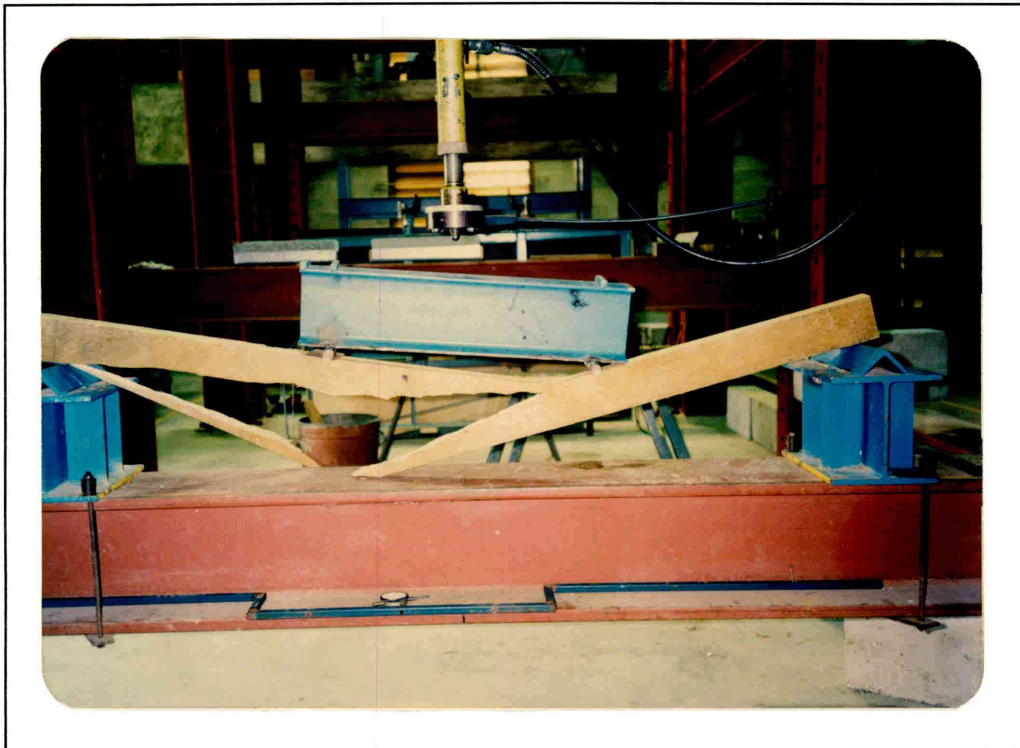
Photo 20: Example of bending failure (sample 14c), Feb 1993 (Y002/6)
