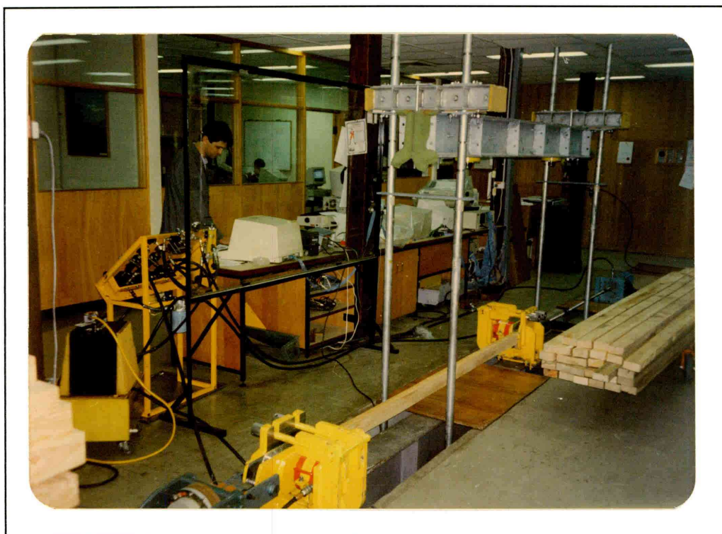
Photo 10: Tensile testing rig at NSW State Forest's Research Division, Pennant Hills (460366/27)
