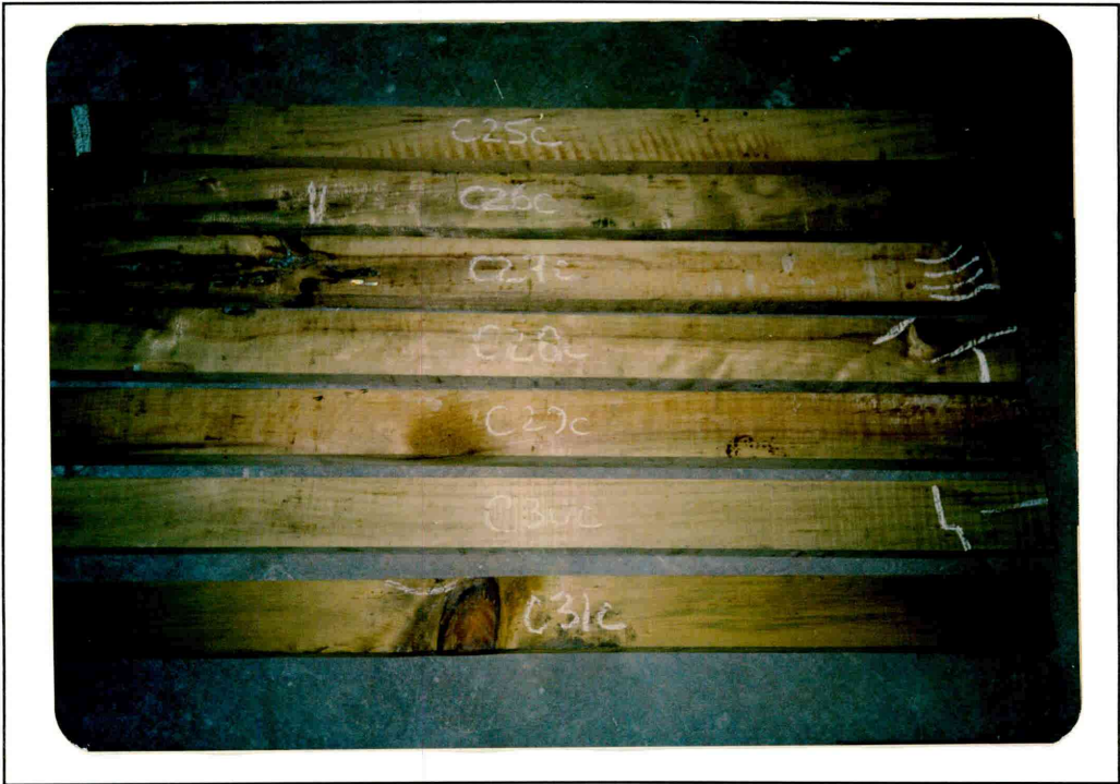
Photo 25: Compressive strength failures (c25c-c31c treated), Mar 1993 (9934/16)
