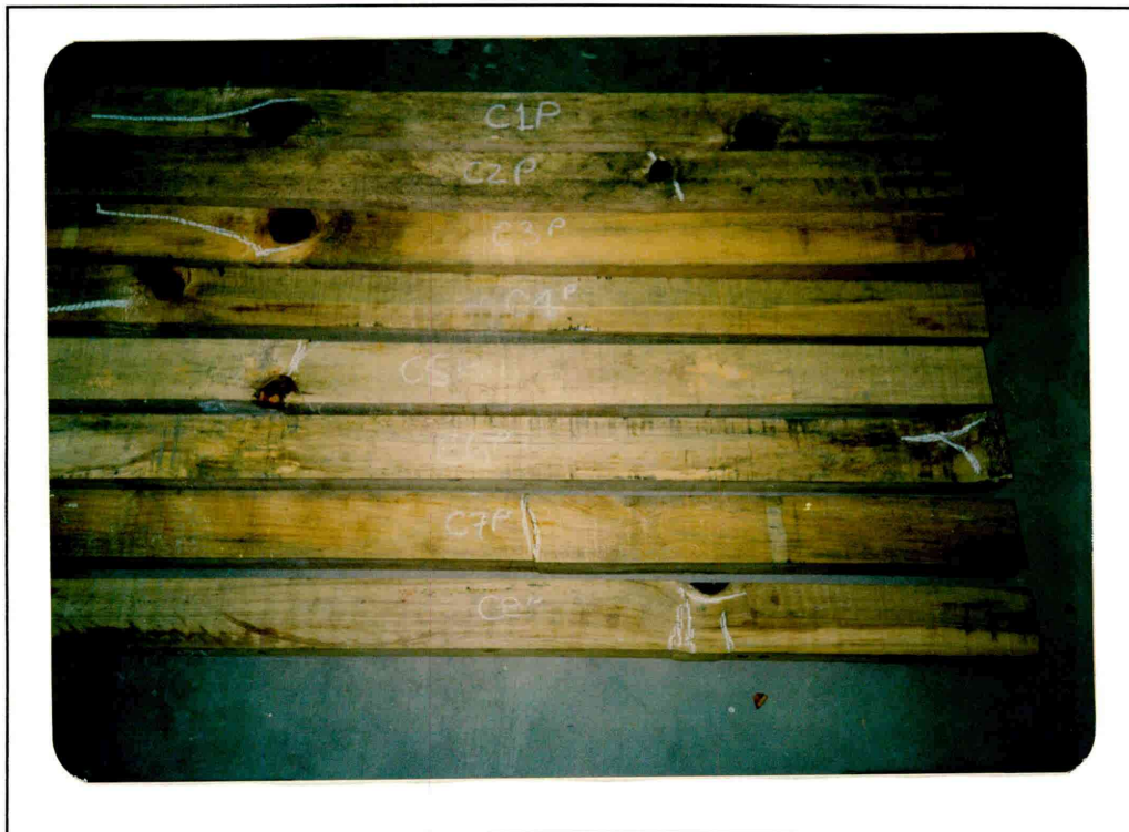
Photo 23: Compressive strength failures (c1p-c8p untreated), Mar 1993 (9934/13)
