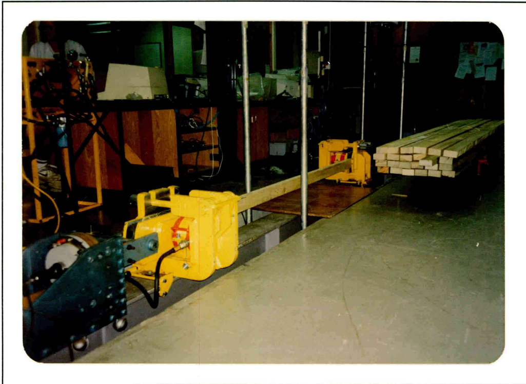
Photo 11: Specimen clamped in tensile test rig at Pennant Hills (460366/24)
