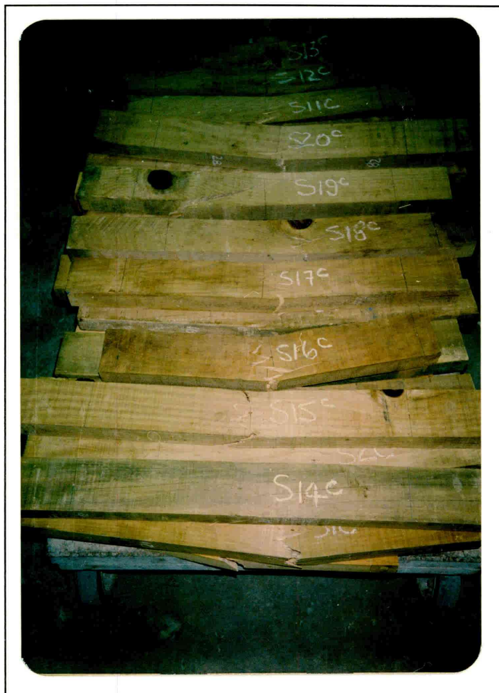
Photo 16: Shear strength tests (s13c to s20c, treated) Feb 1993 (9934/3)
