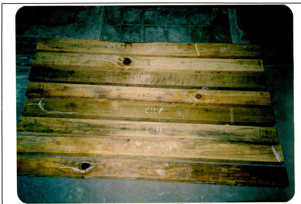
Photo 24: Compressive strength failures (c9p to c16p, untreated), Mar 1993 (9934/10)
