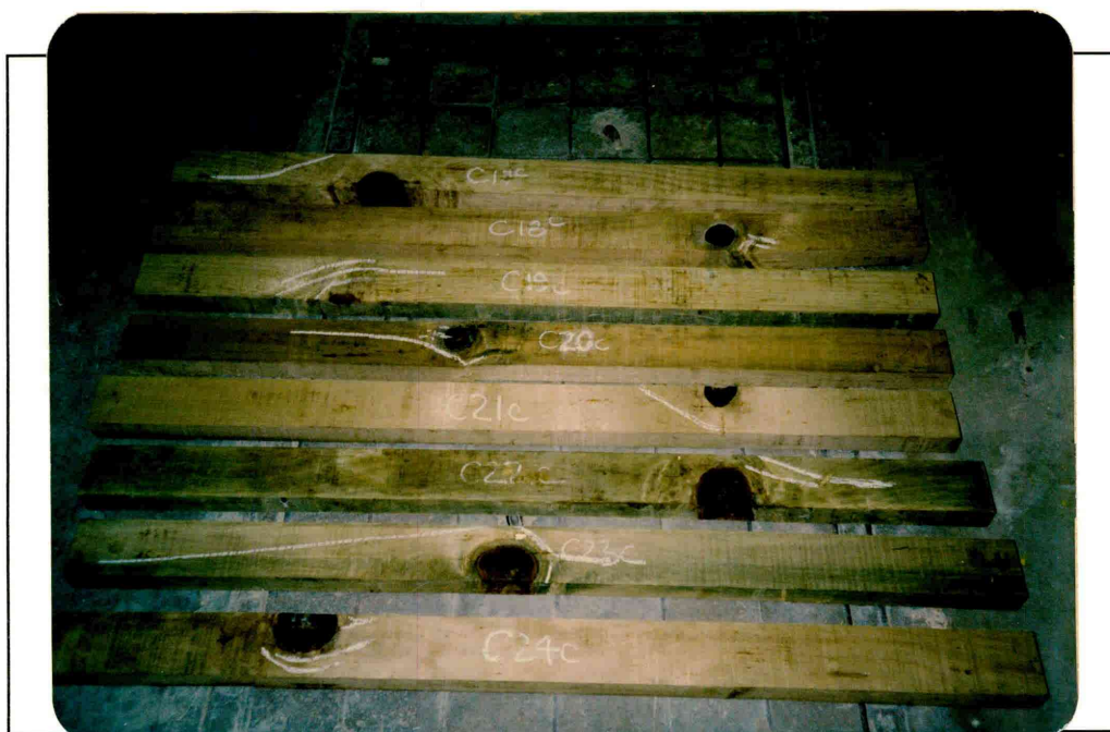
Photo 22: Compressive strength failures (c17c to c24c, treated), Mar 1993 (9934/9)
