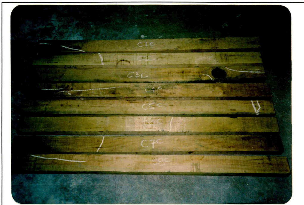
Photo 21: Compressive strength failures (c1c to c8c, treated), Mar 1993 (9934/12)
