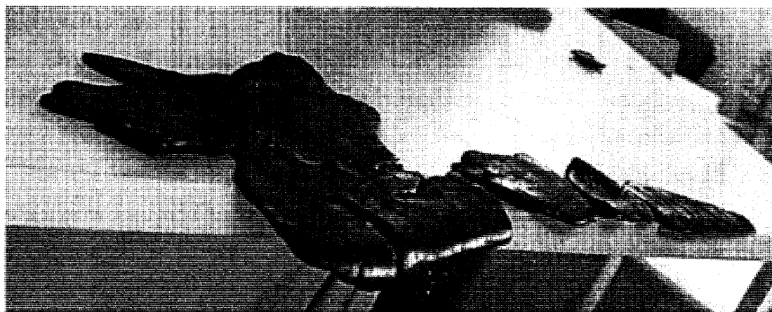
Figure 3.1: Failed bromobutyl rubber found in the slurry mixing tank of AMC.
