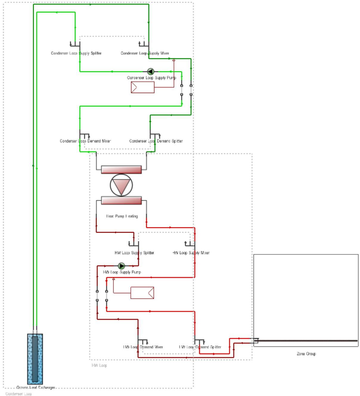
Figure 5.5 Ground Source Heat Pump system diagram considered in the simulation
