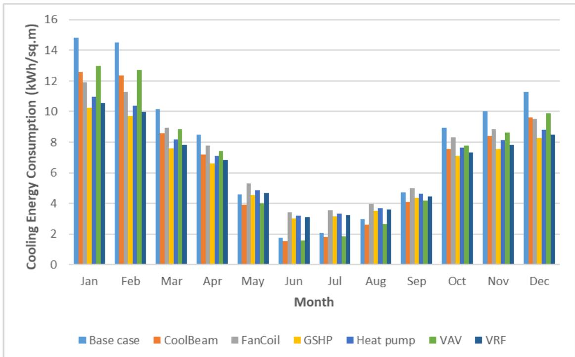
Figure 5.7 Electrical energy consumption using the selective alternative cooling system.
