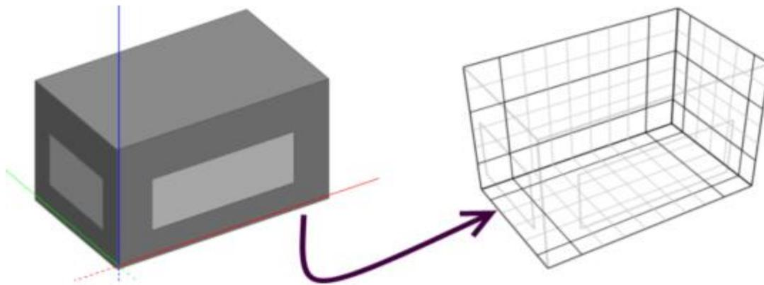
Figure 7.2 Finite volume grid transformation (DesignBuilder Software, 2019)
