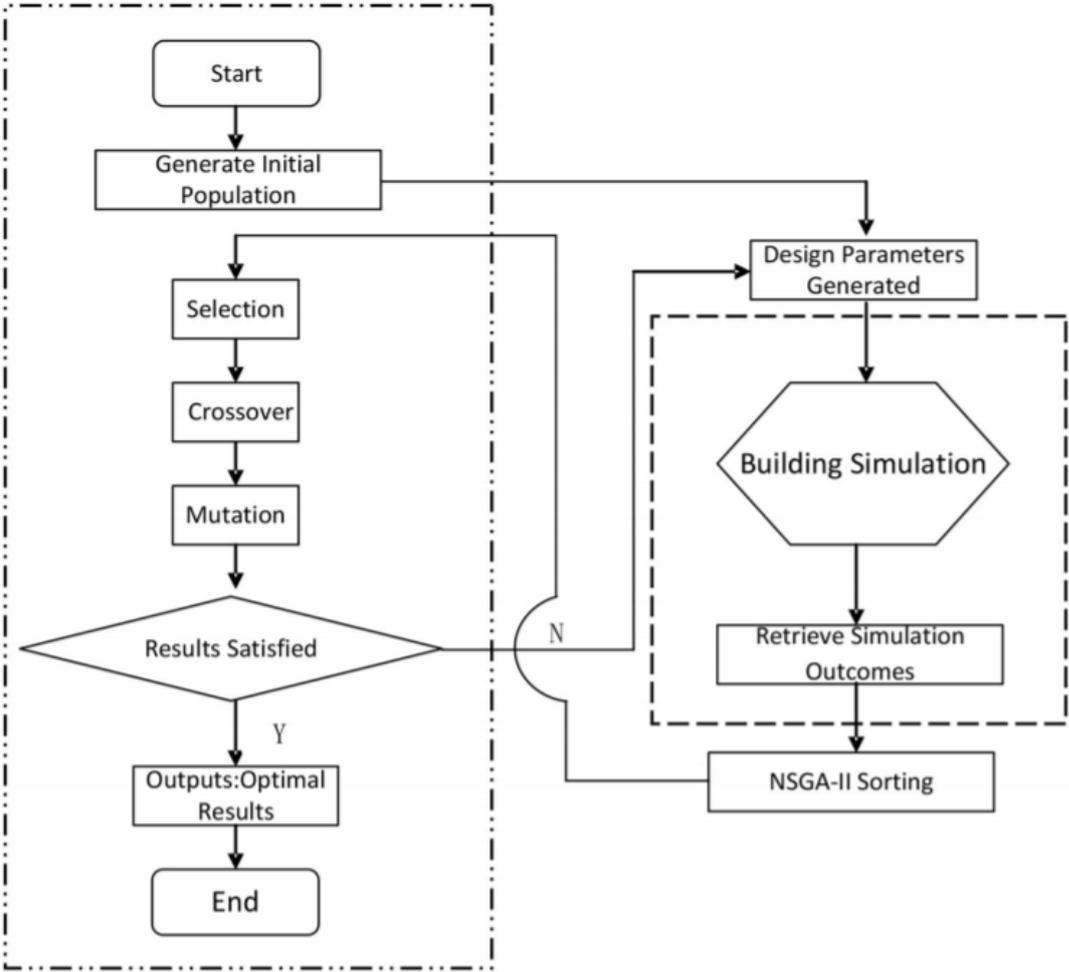
Figure 8.6 Flowchart of the optimisation process following GA (Lin and Yang, 2018)
