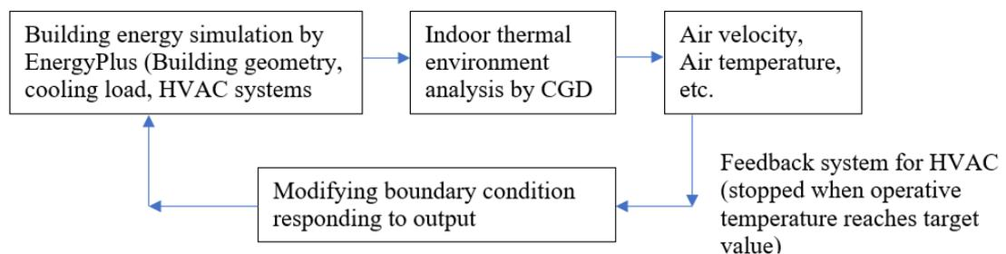
Figure 7.1 CFD Simulation framework for building systems
