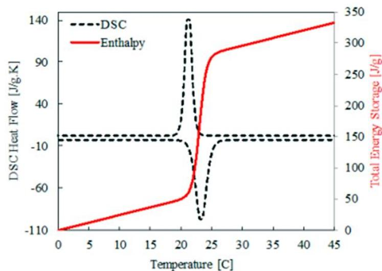
Figure 6.3 Differential scanning calorimeter curve for BioPCM Q23 (Phase Change Energy Solutions, 2019)
