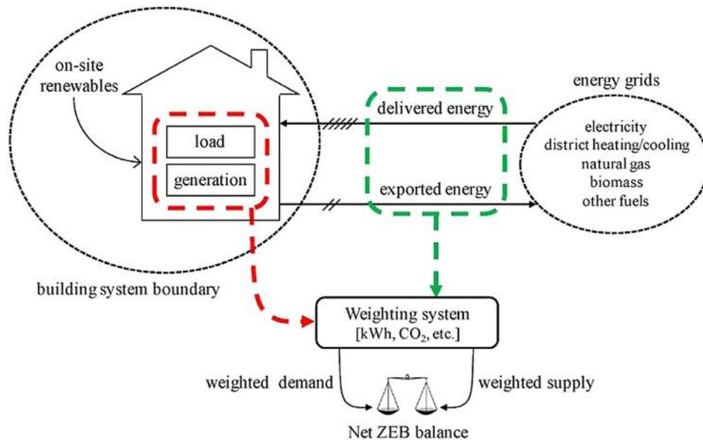
Figure 9.18 A proposed pathway for achieving a balanced zero net energy building (Satori *et al.* 2012)
