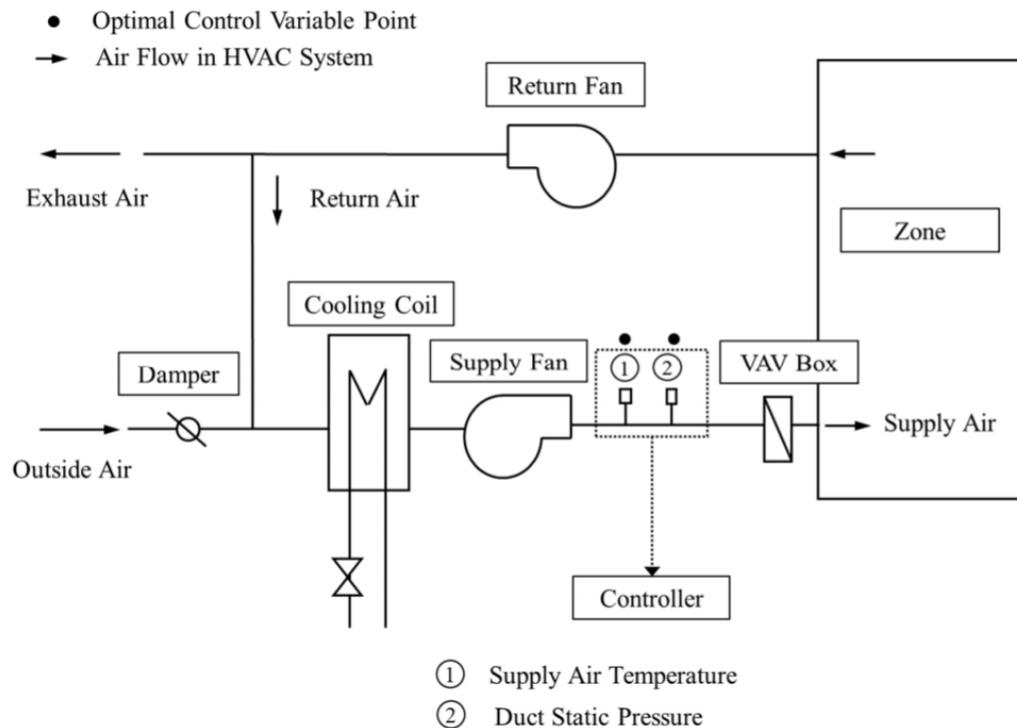
Figure 2.13 Common variable air volume (VAV) air-conditioning system (Seong *et al.* 2019).
