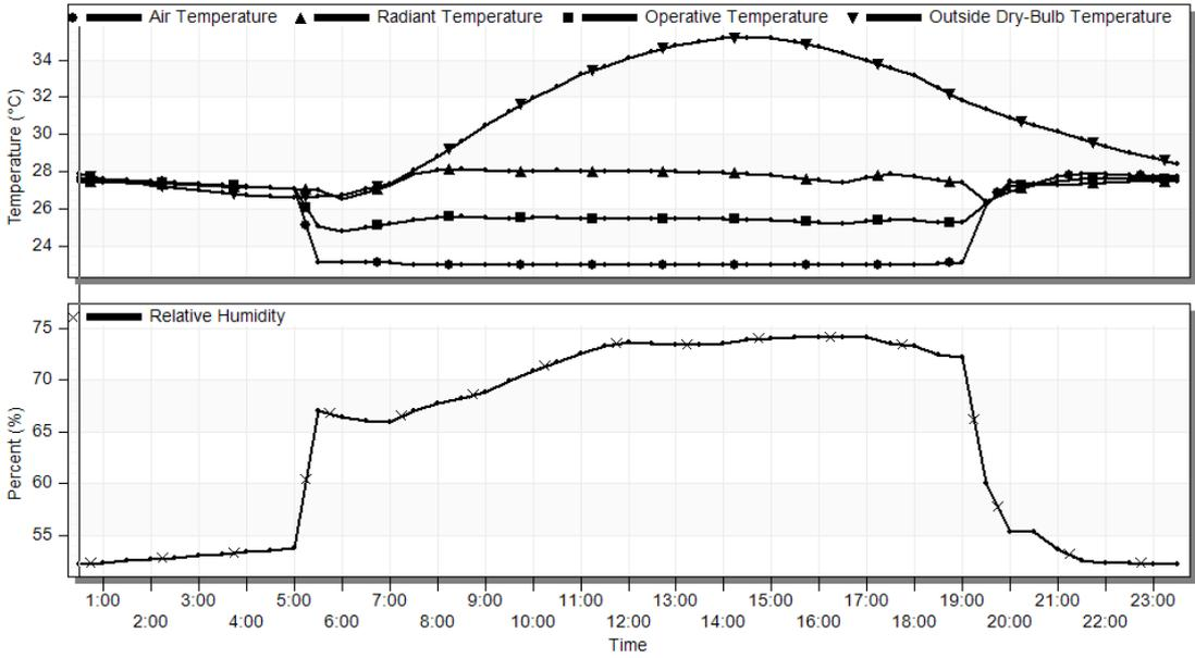
Figure 7.3 Temperature and relative humidity using the base case scenario
