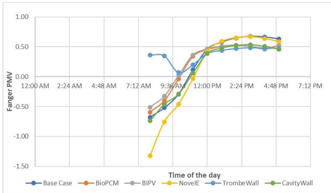
Figure 7.7 Thermal comfort index using the alternative envelope system in winter
