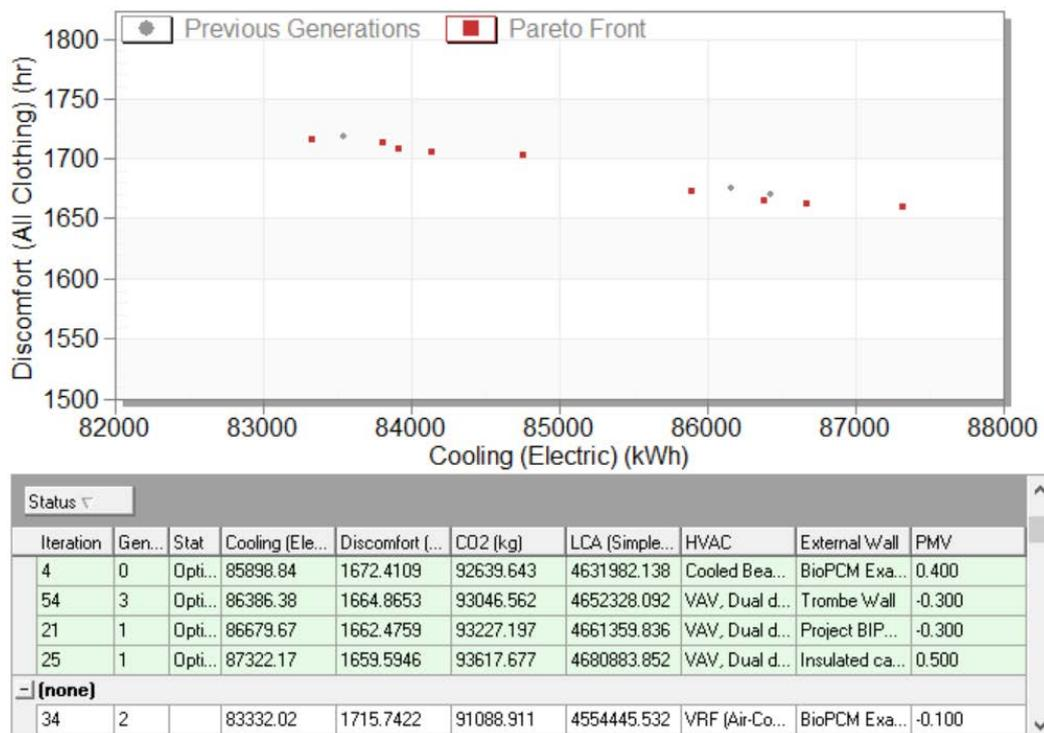
Figure 9.17 Optimizing cooling energy consumption and discomfort hours considering possible 2.0 °C temperature increase in future
