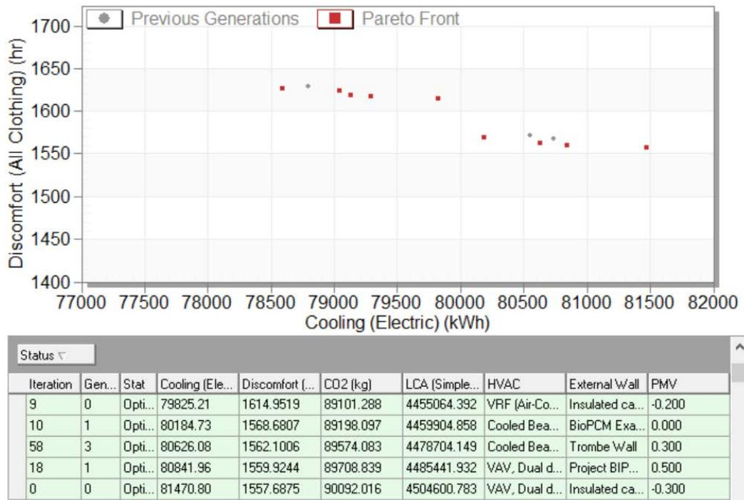
Figure 9.16 Optimizing cooling energy consumption and discomfort hours considering potential 1.5 °C temperature increase in future
