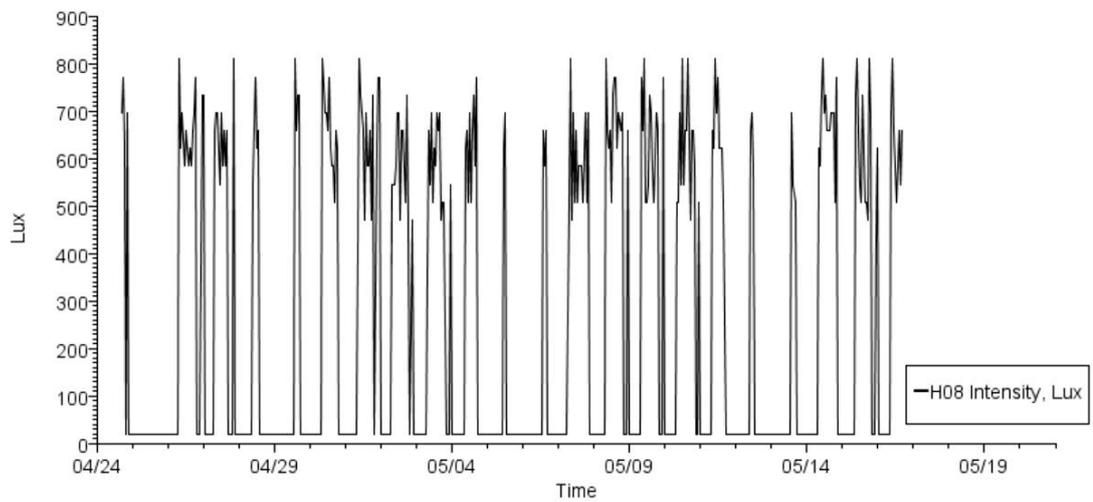
Figure 3.11 Recorded lighting intensity value (as extracted from the datalogger using HOBOWare)
