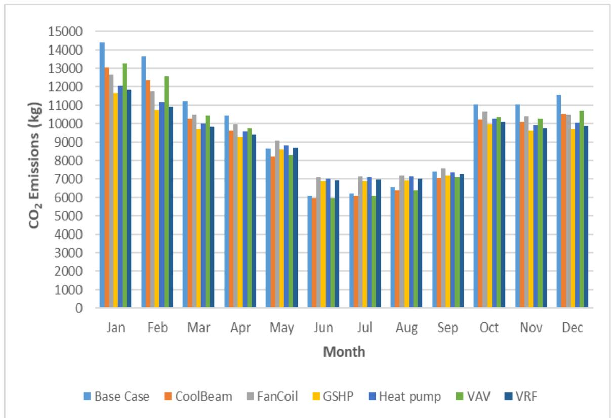
Figure 5.10 CO<sub>2</sub> emission reduction under the selected alternative cooling system.
