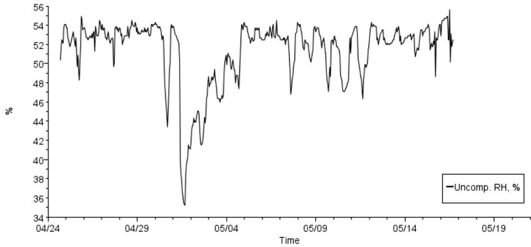
Figure 3.10 Recorded humidity profile (as extracted from the datalogger using HOBOWare).
