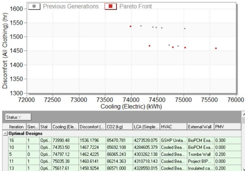
Figure 9.15 Optimizing cooling energy consumption and discomfort hours considering potential 1.0 °C temperature increase in future
