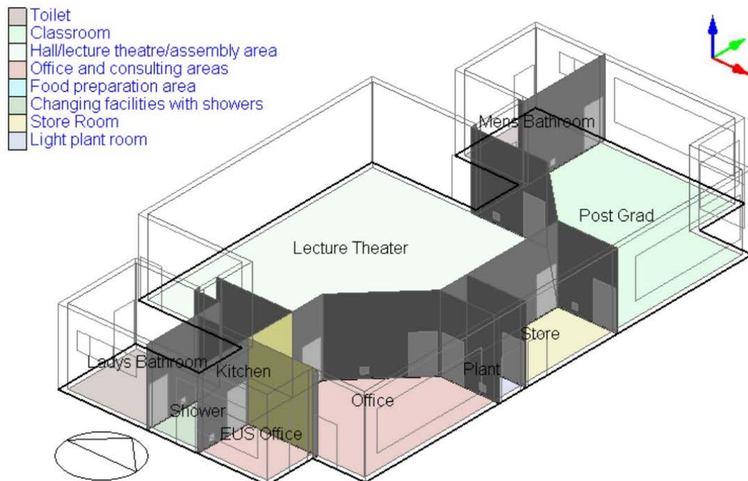
Figure 4.12 Representation of the thermal modelling zones (ground floor).
