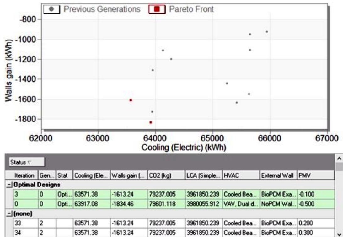
Figure 8.8 Optimising cooling energy consumption and heat gain through the wall.
