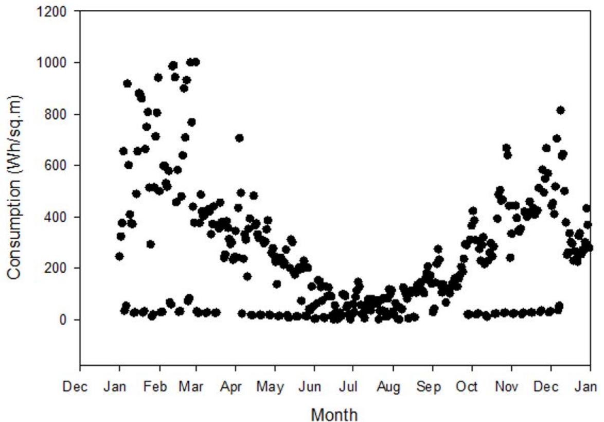
Figure 3.14: HVAC electricity usage pattern.
