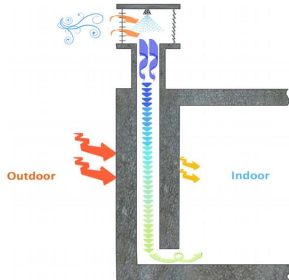
Figure 2.12 Standard representation of the aerated cavity wall with evaporator (Alaidroos and Krarti, 2016).
