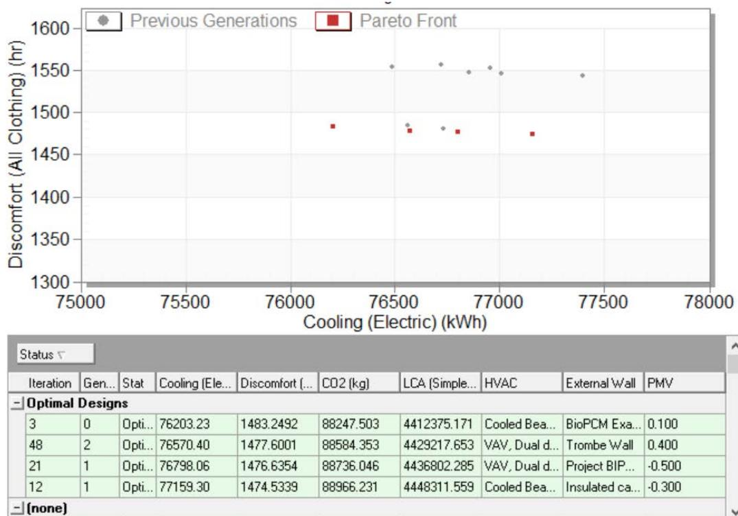
Figure 9.13 Optimizing cooling energy consumption and discomfort hours considering the potential average future weather condition
