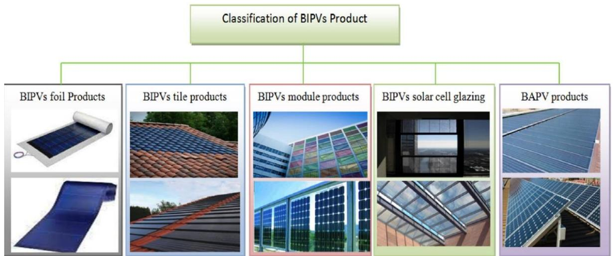
Figure 2.9 Categories of BIPV products (Alim *et al.*, 2019).
