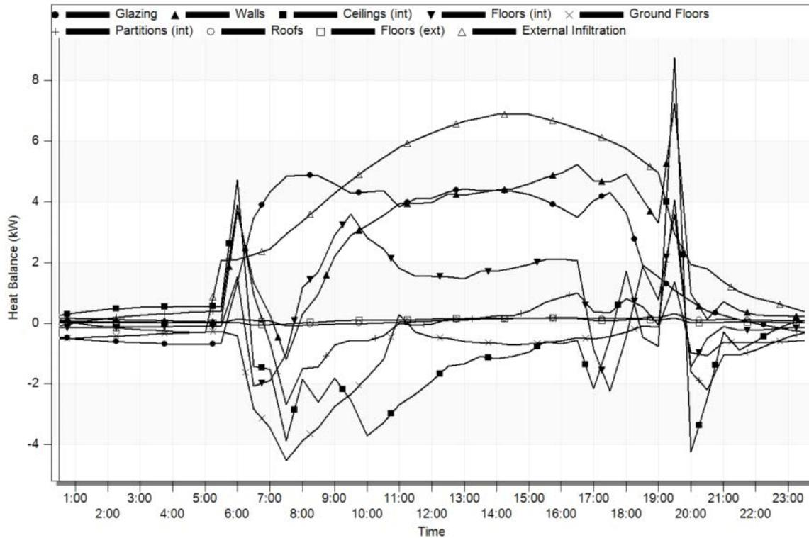
Figure 4.19 Heat balance via ventilation and envelope in cooling design.
