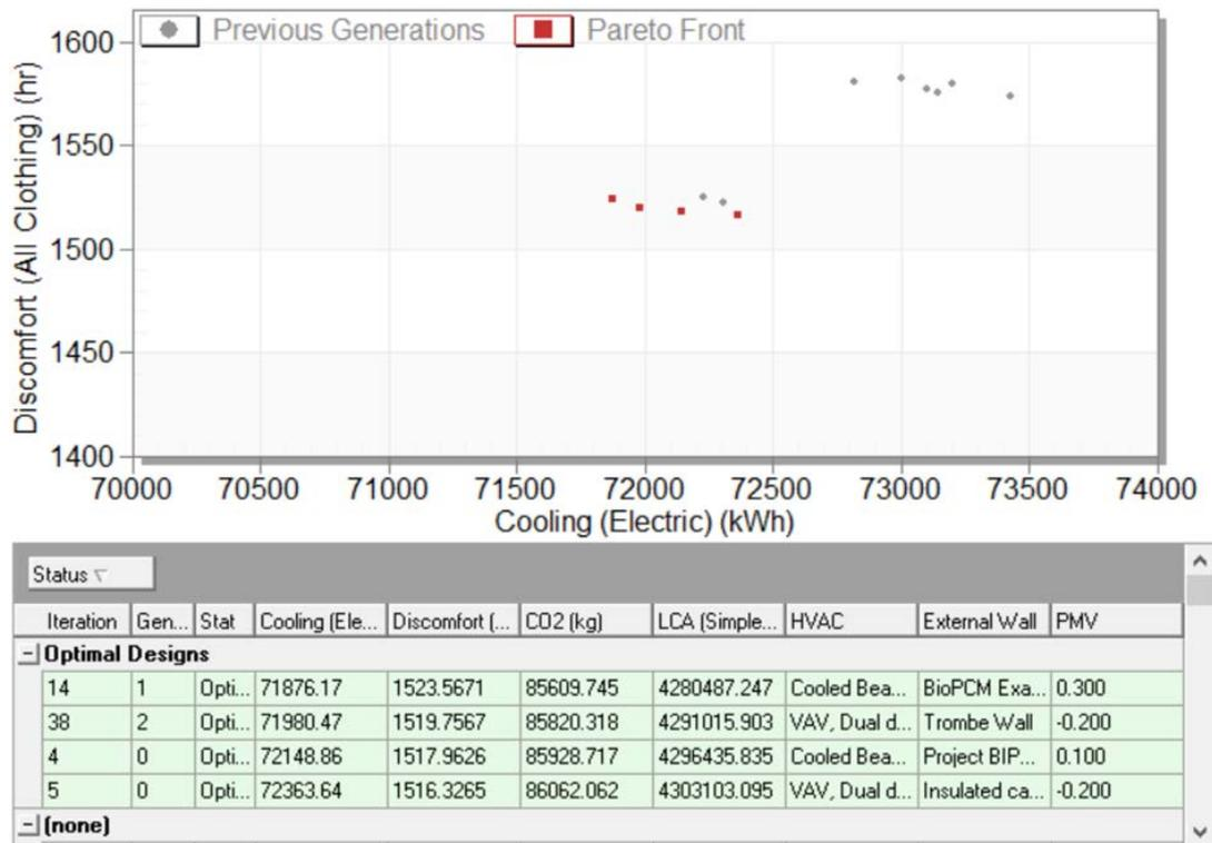
Figure 9.14 Optimizing cooling energy consumption and discomfort hours considering potential 0.5 °C temperature increase in future
