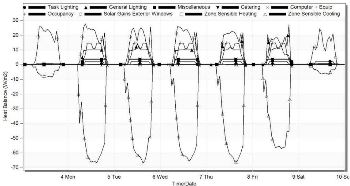
Figure 4.22 Indoor heat balance and cooling load in the representative summer week
