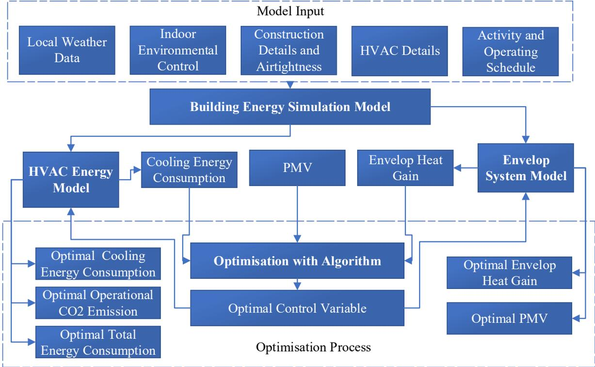
Figure 8.7 Energy and comfort analysis design for building a HVAC and envelope system utilising genetic algorithms.
