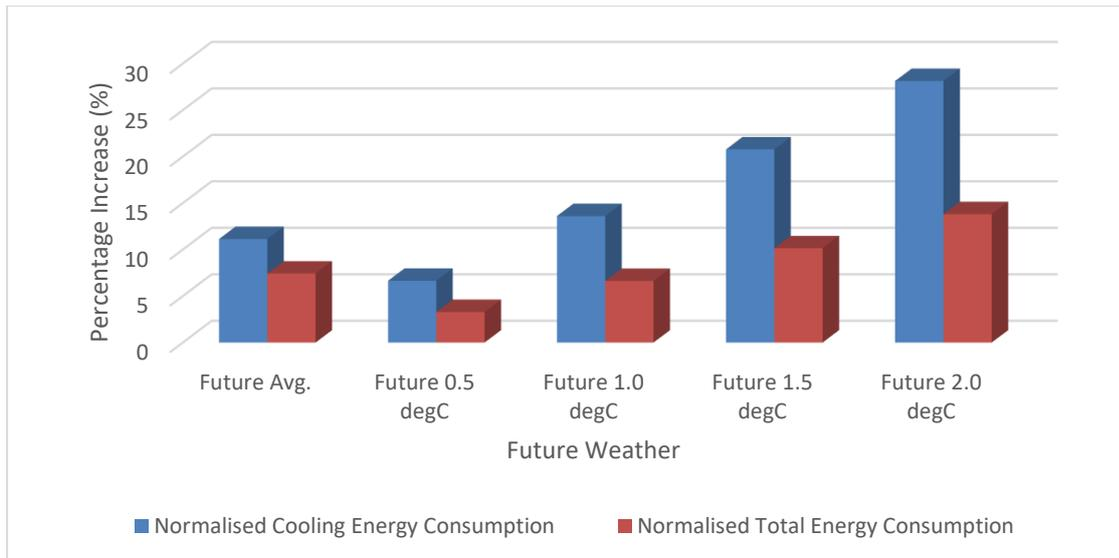
Figure 9.12 Assessment of increased normalised yearly cooling and overall energy consumption considering the future potential average weather condition
