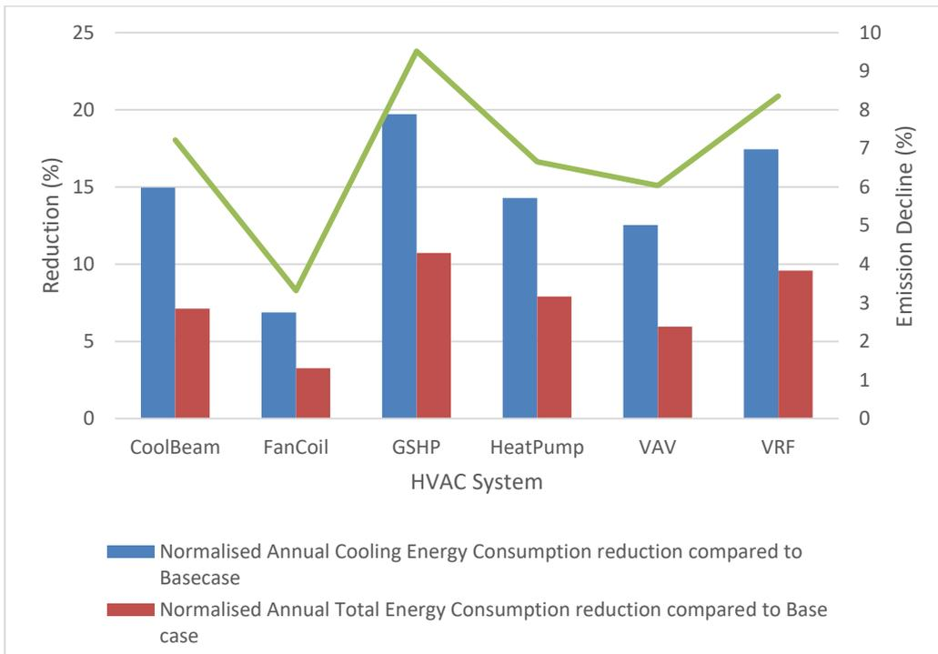
Figure 5.12 Reduction in normalised energy consumptions and CO<sub>2</sub> emissions.
