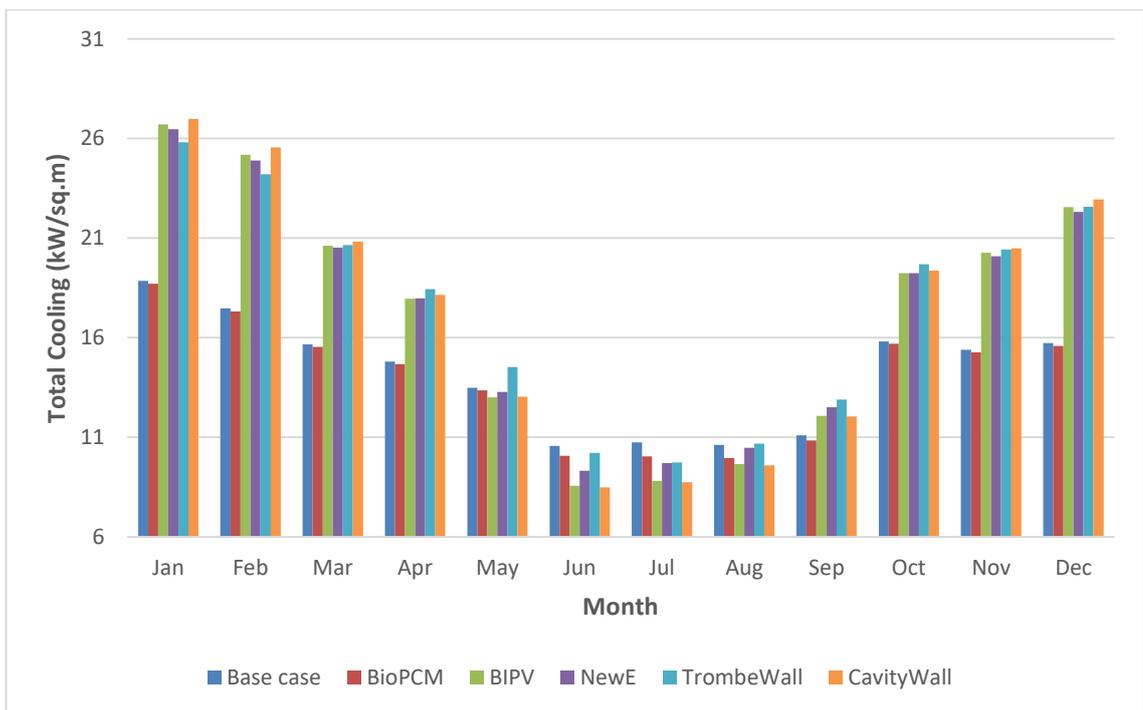
Figure 6.8 Total cooling load using alternative envelope systems
