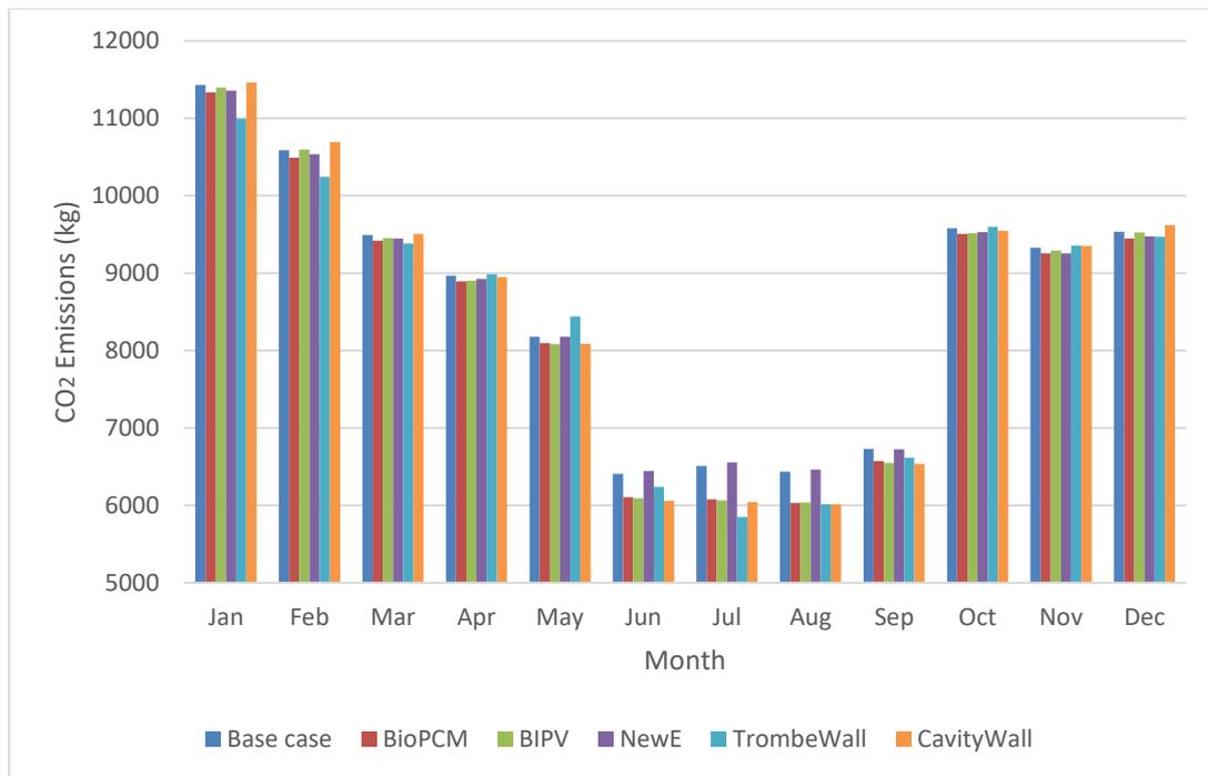
Figure 6.6 Operational CO<sub>2</sub> emission profile under alternative envelope systems
