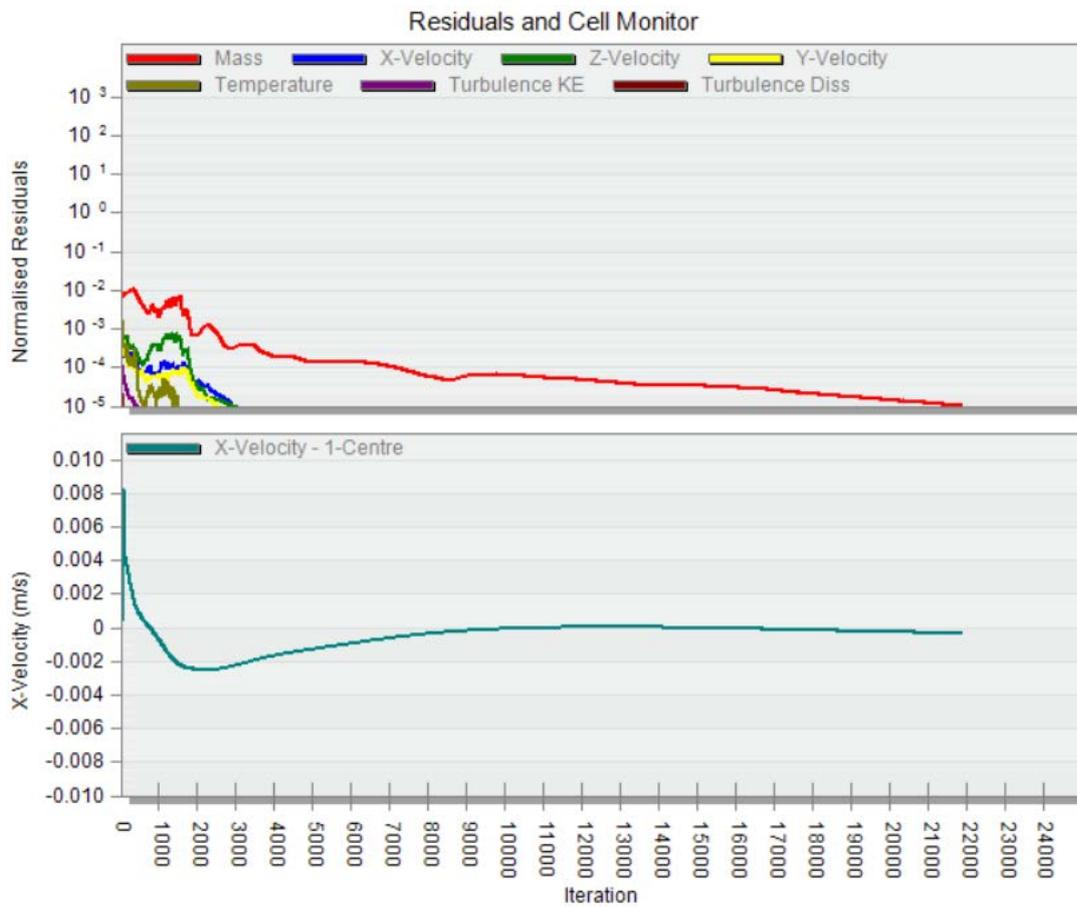
Figure 7.14 CFD converged solution considering mass, velocity, and temperature
