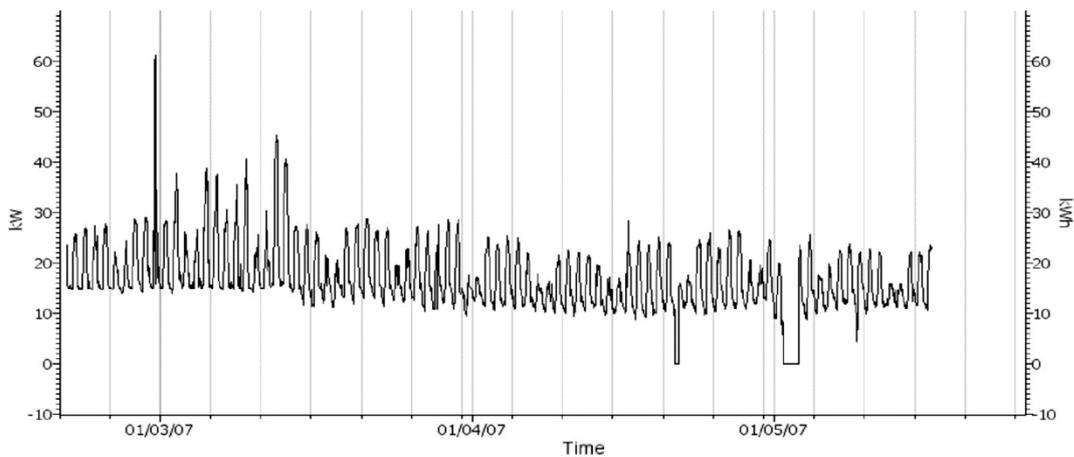
Figure 3.13: Chiller power demand and electricity consumption profile. (as extracted from the datalogger using HOBOWare)
