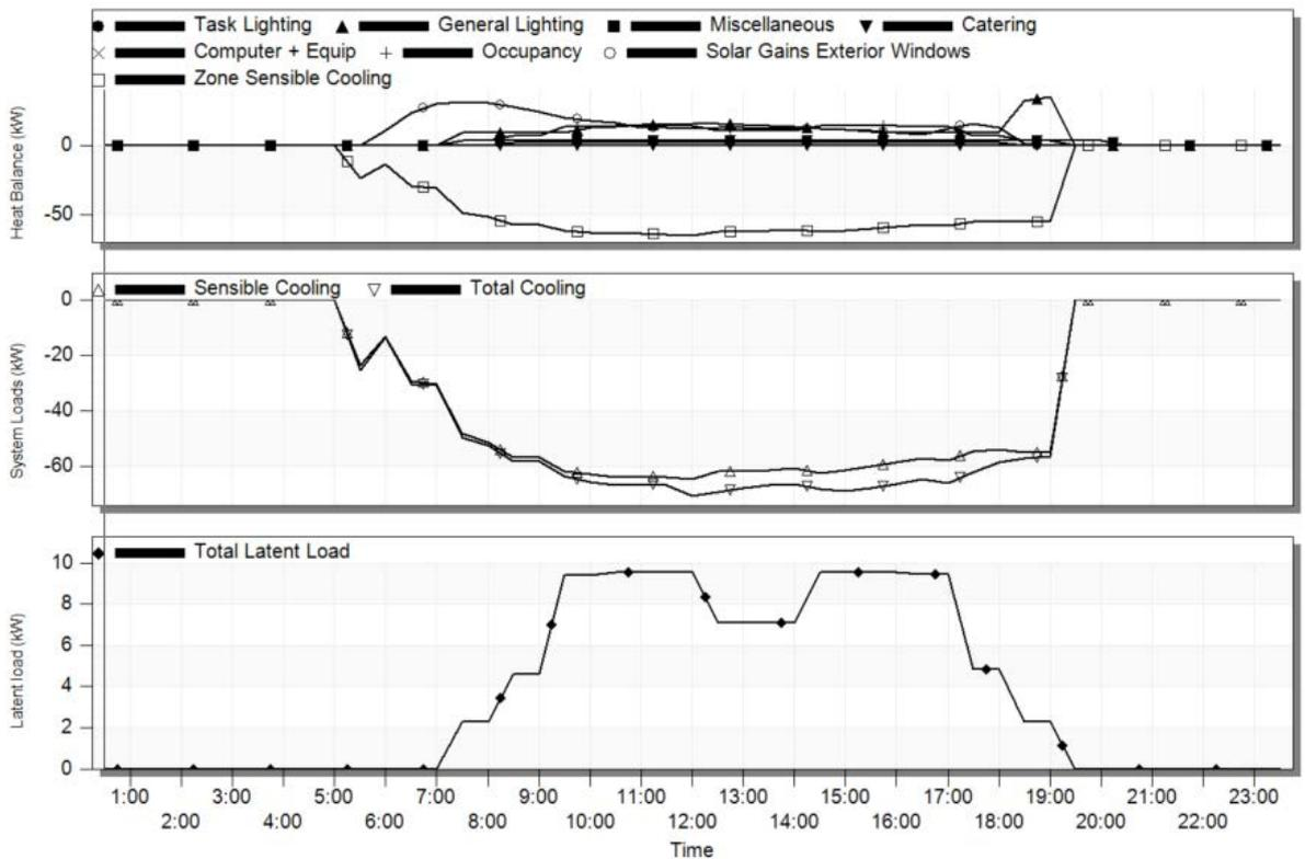
Figure 4.18 Heat gain and losses in cooling estimate.
