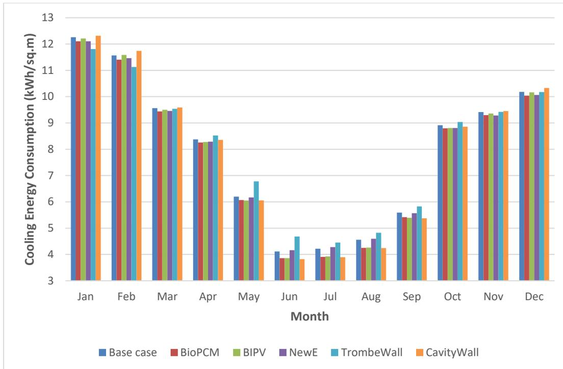
Figure 6.4 Cooling energy consumption profile under alternative envelop systems
