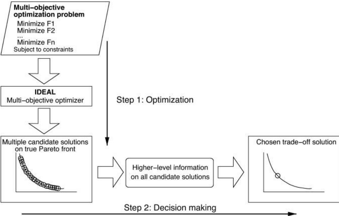
Figure 8.3 Multi-objective optimisation procedure (Justesen, 2010)
