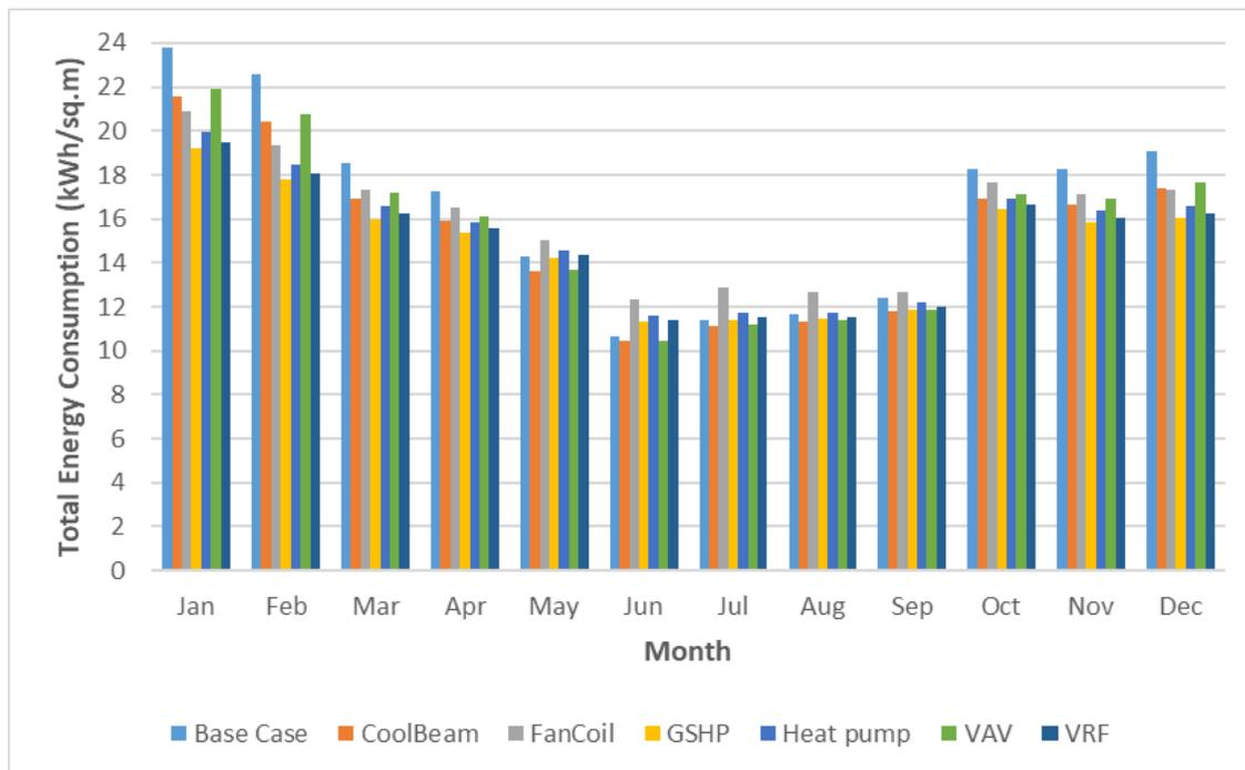
Figure 5.9 Whole building energy consumption under the selective alternative cooling system
