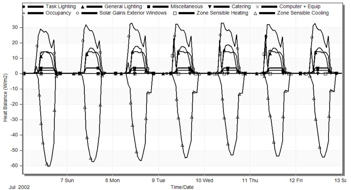
Figure 4.23 Indoor heat balance and cooling load in the representative winter week.
