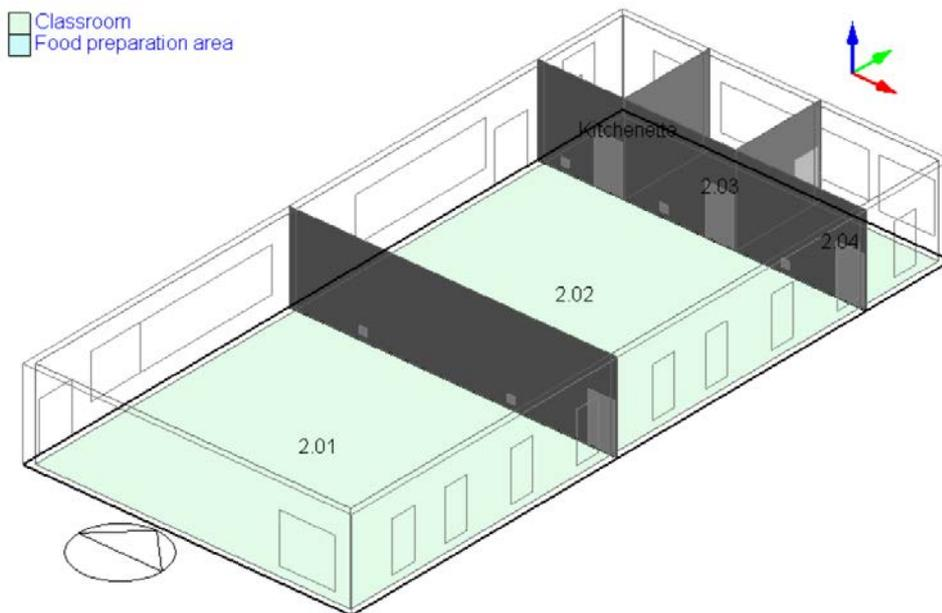
Figure 4.14 Representation of the thermal modelling zones (second floor)
