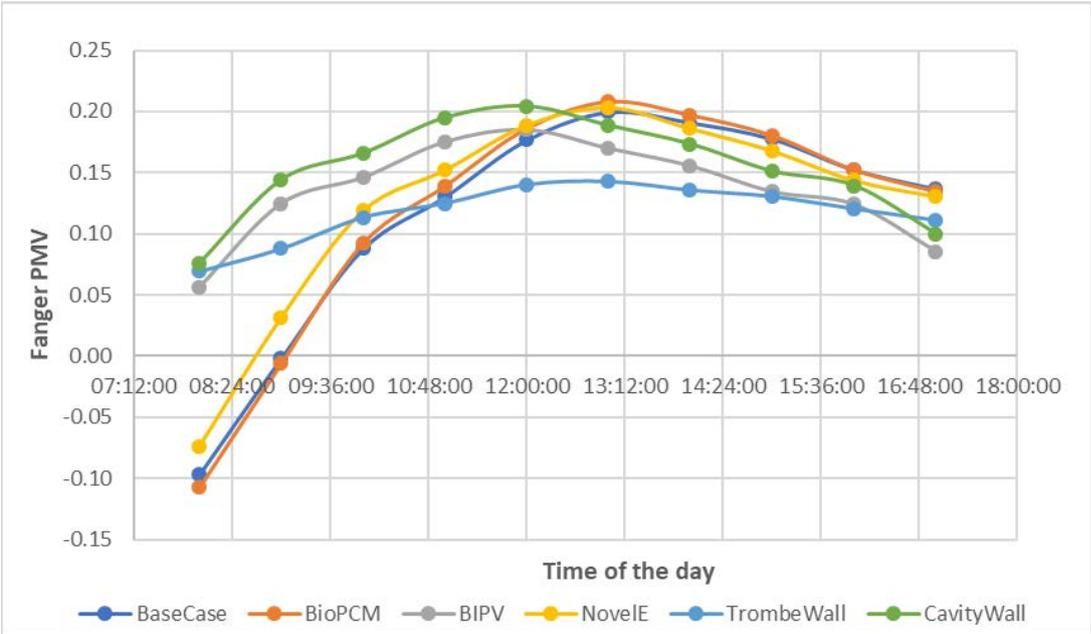
Figure 7.6 Thermal comfort index using the alternative envelope system in summer
