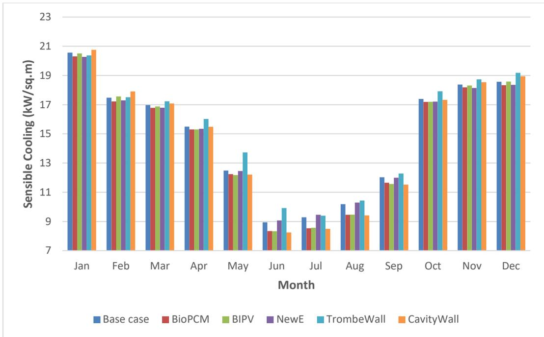
Figure 6.7 Sensible cooling load using alternative envelope systems
