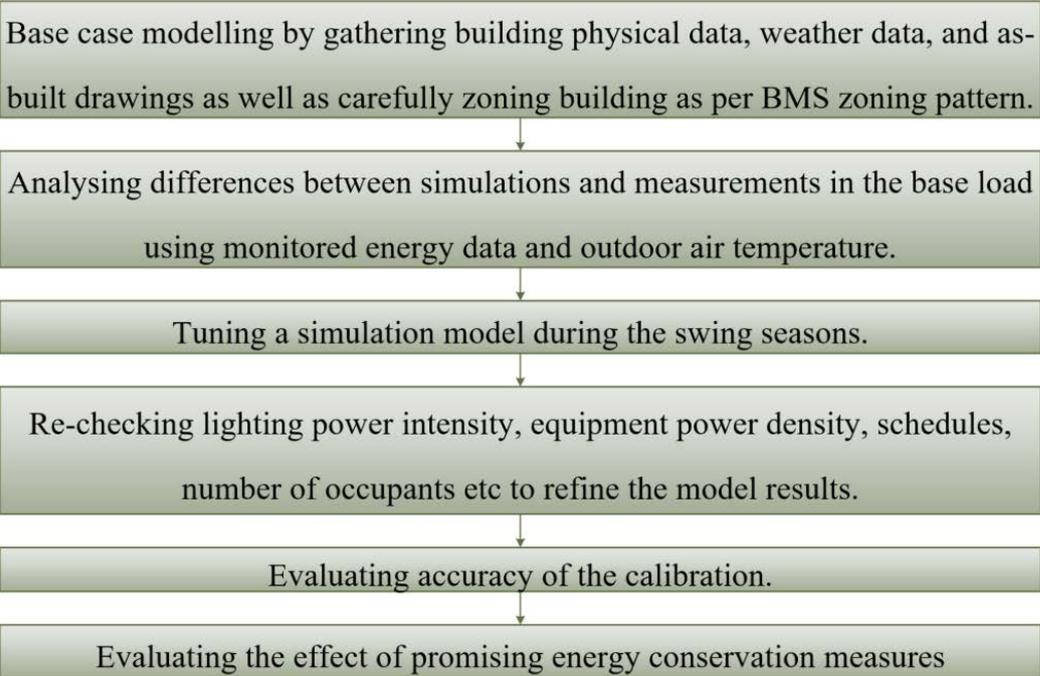
Figure 4.30 Calibration process of the modelled results.
