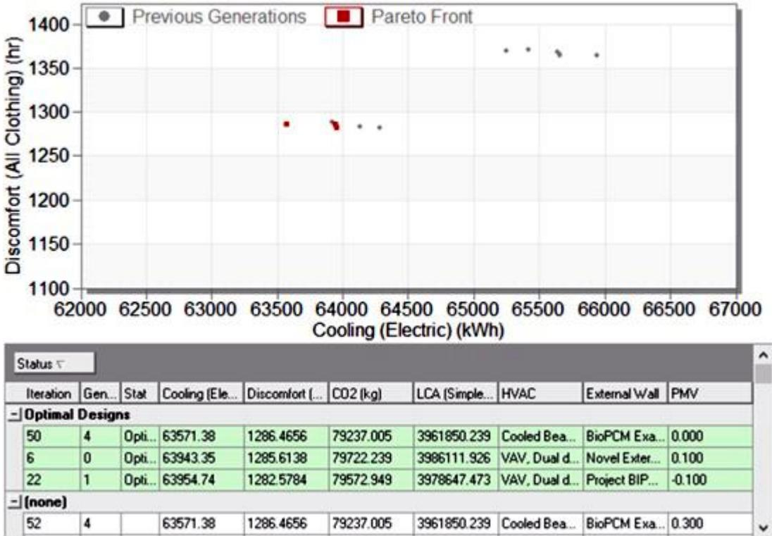
Figure 8.9 Optimising cooling energy consumption and discomfort hours.
