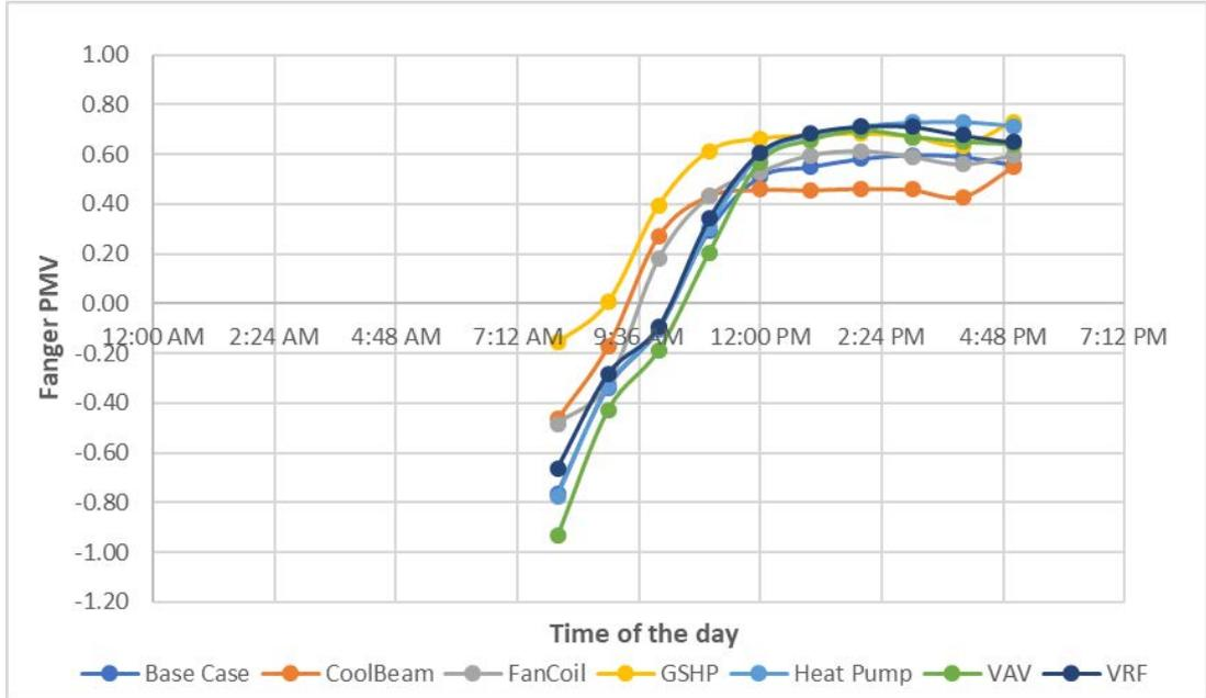
Figure 7.9 Thermal comfort index using the alternative HVAC systems in winter
