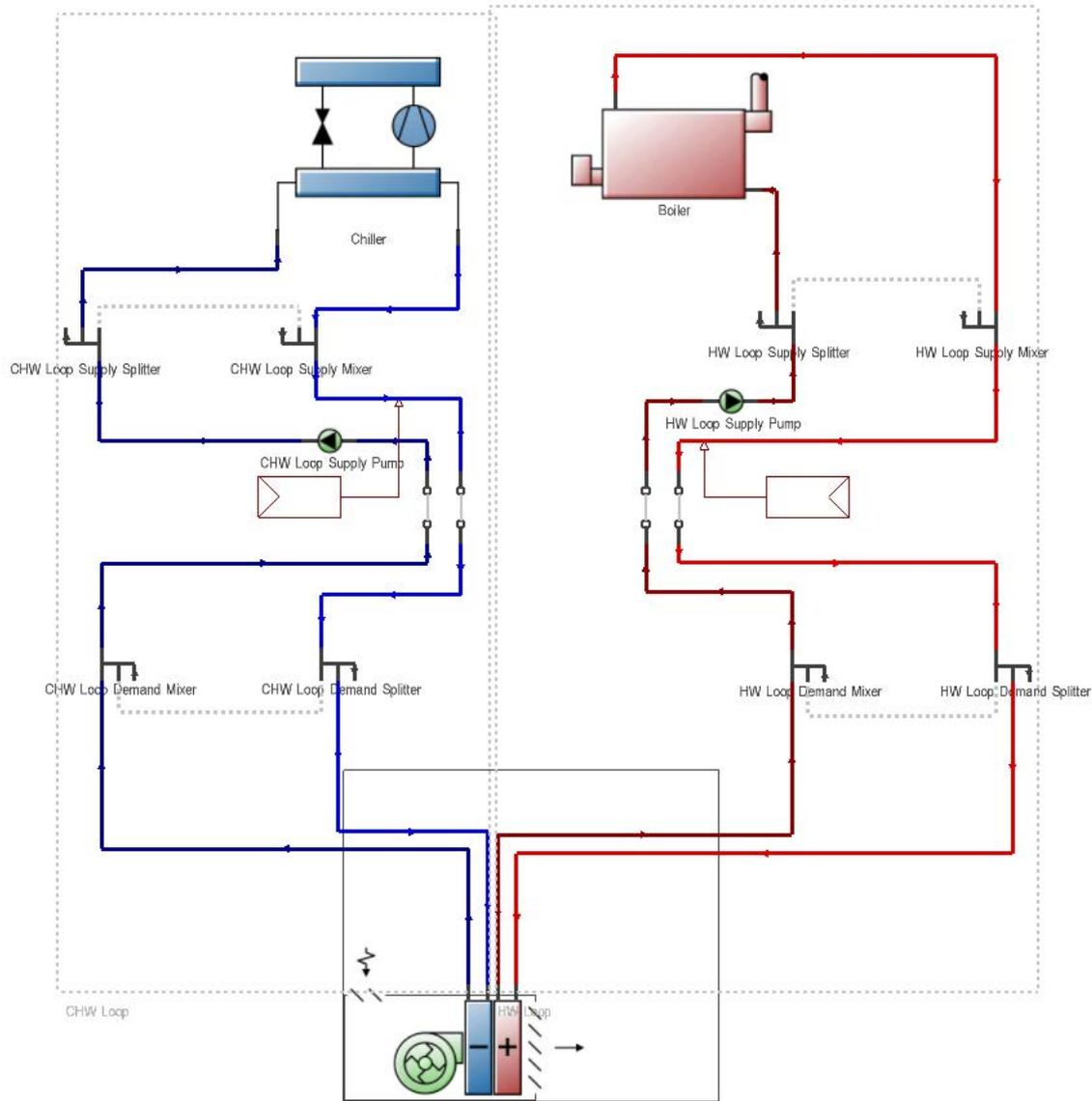
Figure 5.4 Fan Coil Unit system diagram considered in the simulation.
