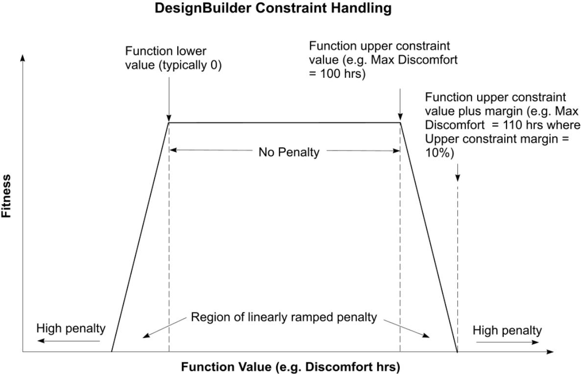
Figure 8.5 DesignBuilder constraint handling (DesignBuilder Software, 2019)
