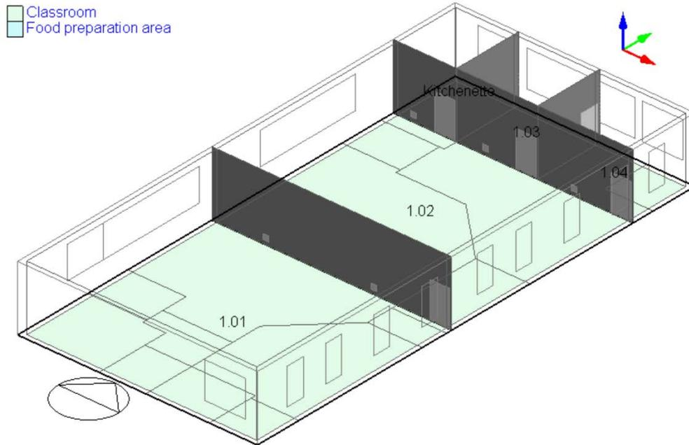
Figure 4.13 Representation of the thermal modelling zones (first floor)
