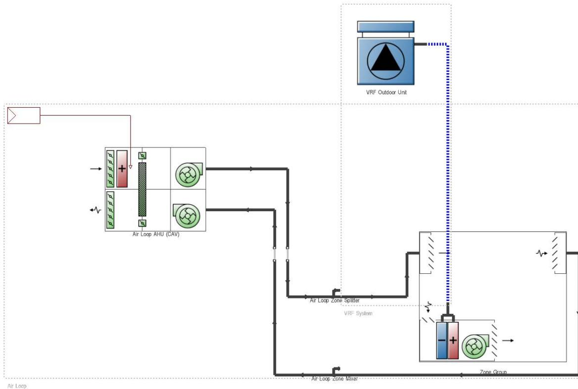
Figure 5.3 Illustration of the VRF system considered in the simulation.
