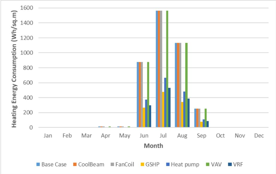
Figure 5.8 Heating energy consumption under a selective alternative cooling system.
