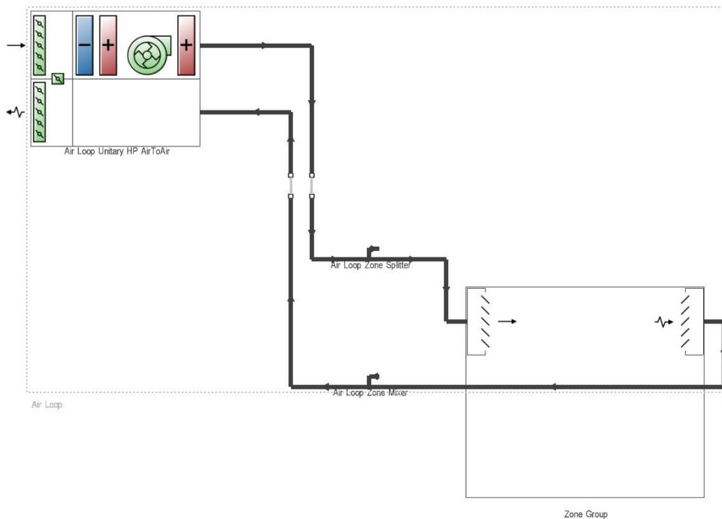
Figure 5.2 PTHP system diagram considered in the simulation.
