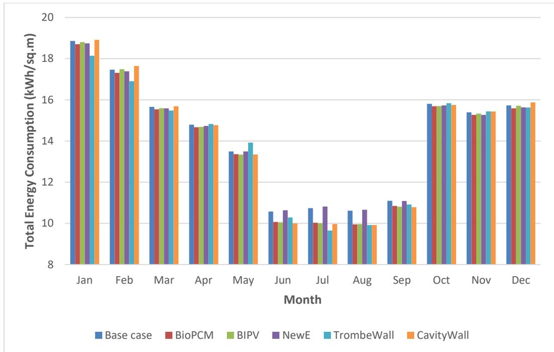
Figure 6.5 Total electricity consumption profile under alternative envelope systems
