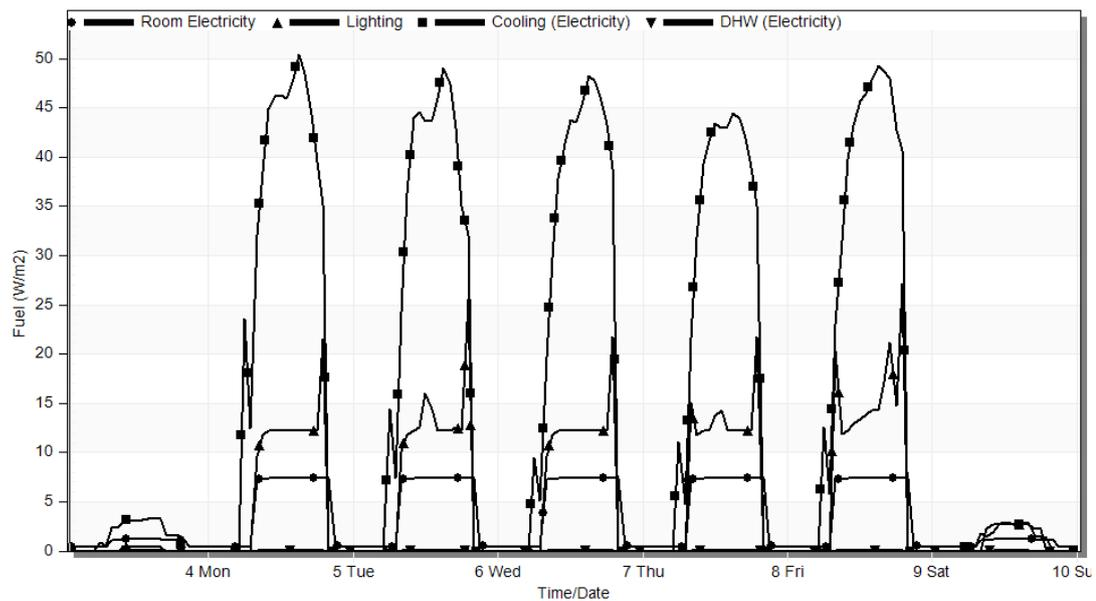
Figure 4.26 Electrical energy usage breakdown in a summer week.
