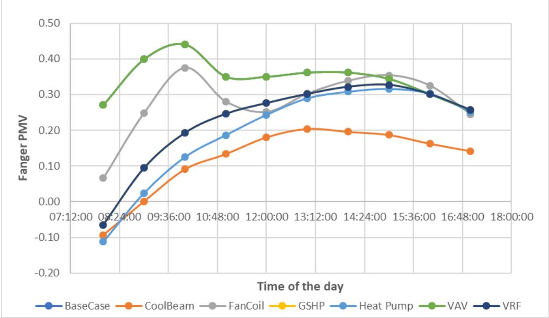
Figure 7.8 Thermal comfort index using the alternative HVAC systems in summer
