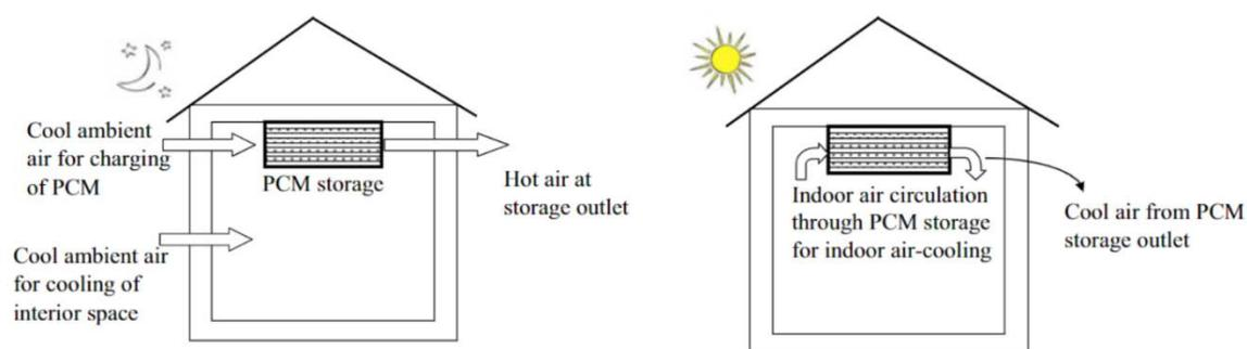
Figure 2.8 Charging and discharging processes using PCM (Waqas and Din 2013).
