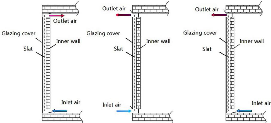
Figure 2.11 Trombe wall in area heat up approach; outdoor flow approach and cross exposure to air approach respectively (Hong *et al.* 2019).
