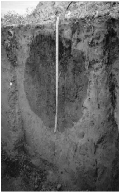
Figure 2.2.1 Position of the wetting front after 10 h irrigation applied at 1.7 \text{ l h}^{-1} from simulated emitter installed at a depth of 0.30 m in a loamy soil (Source: Battam et al. , 2003).
