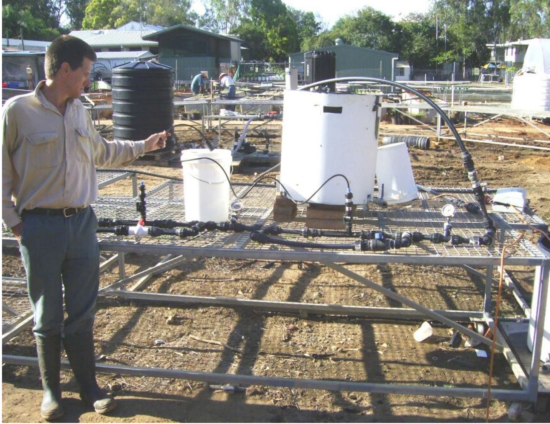
Figure 3. 4 The position of the chemical injector venturi in the irrigation system.
