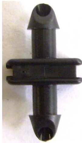
Figure 3. 2 An asymmetric connector. These connectors are inserted into irrigation pipe with the high end upstream.
