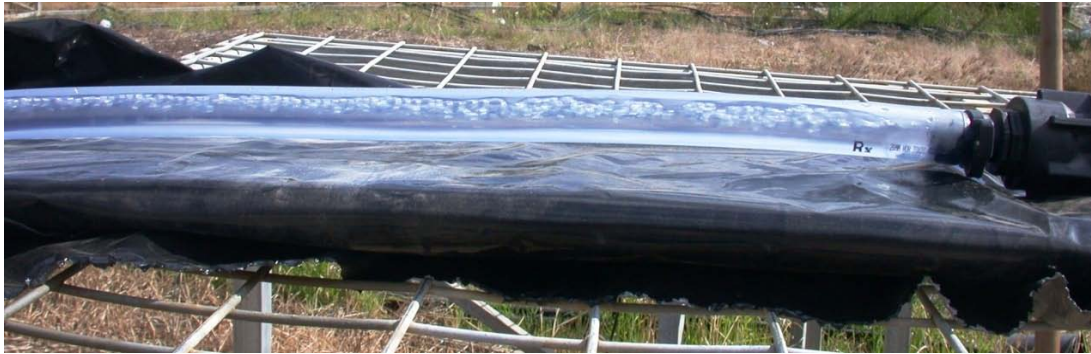
Figure 3. 44 Formation of air bubbles in an irrigation pipe immediately after a venturi.
