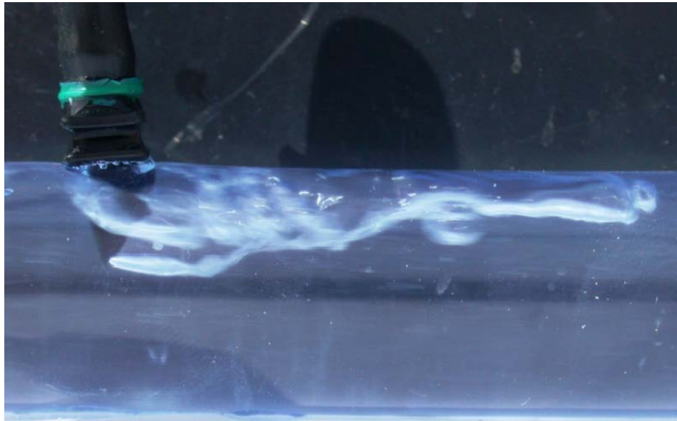
Figure 3. 47 The turbulent flow at the vicinity of an asymmetric connector.
