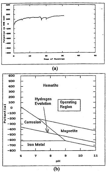
Figure 2 (a) Corrosion potential-time data for a Queensland power station (b) The data displayed on a Pourbaix diagram; illustrating that the system is in a "safe" operating mode.
