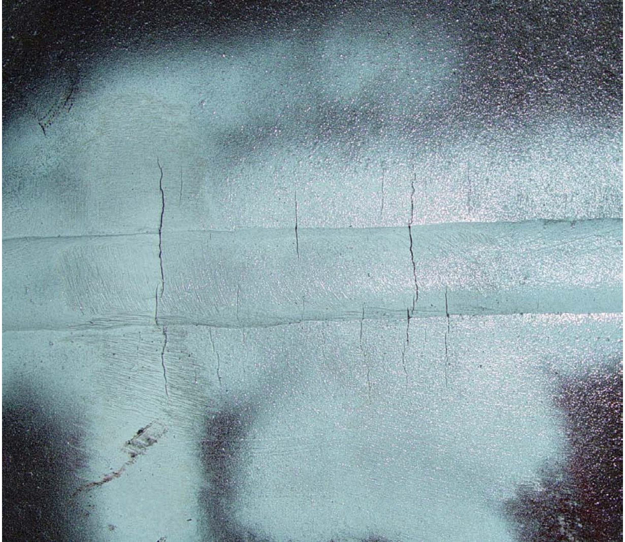
Figure 3 Transverse cracking in seam welds.
