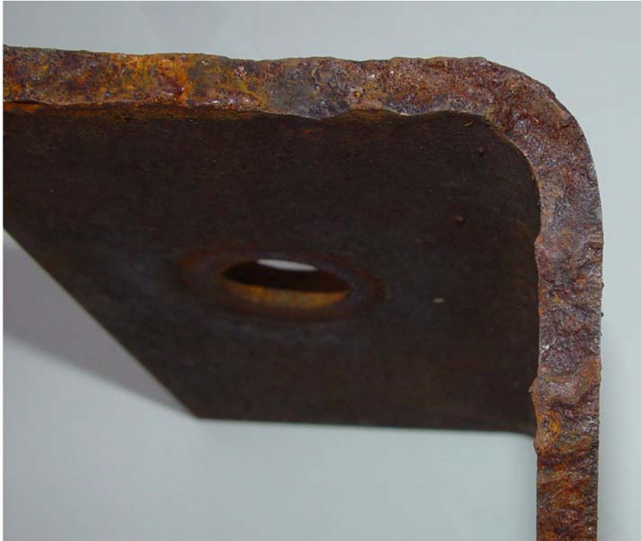
Figure 2 Lifter showing the cracked lugs. These lugs had been welded to the shell and had fractured through the HAZ of the weld.
