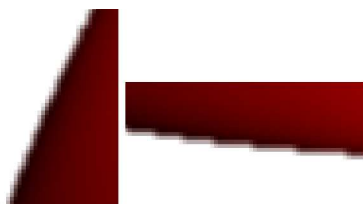
Figure 2.6: Edge blur is satisfactory for moderate slopes in either direction but not for steep or shallow edges.
