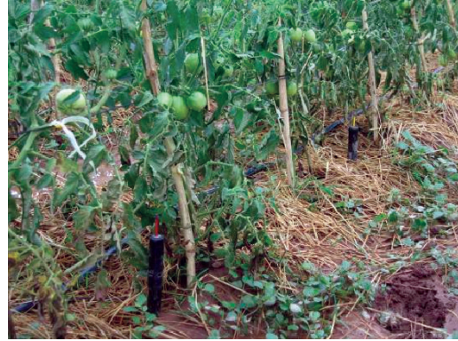
Figure 26. Soil tensiometer placement in hot pepper drip irrigation field trial plot (a) and Fullstop Wetting Front Detector on drip irrigated tomato crop (b).
