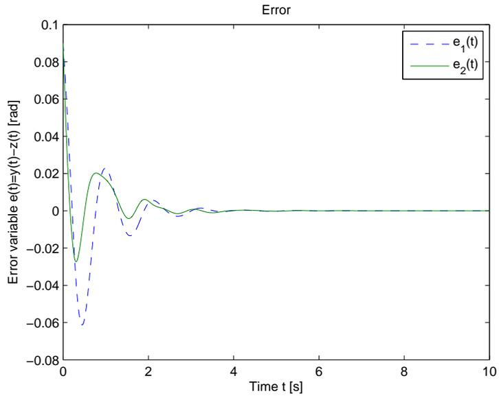
Fig. 9. Simulation result for error system with the feedback controller gain derived by Proposition 3,  $\tau = 0.24$ , and  $A = 0.3 \text{ kg mm}$ ,  $B = 0.5 \text{ kg mm}$ ,  $C = 0.2 \text{ kg mm}$ ,  $D = 0.4 \text{ kg mms-1}$ ,  $r = 0.11559633 \text{ kg m}$ ,  $R_0 = 6378000 \text{ m}$ ,  $g = 9.8 \text{ ms-2}$ ,  $F = 3.4 \text{ N}$ ,  $\omega = 1.8 \text{ rad ms-1}$ .
