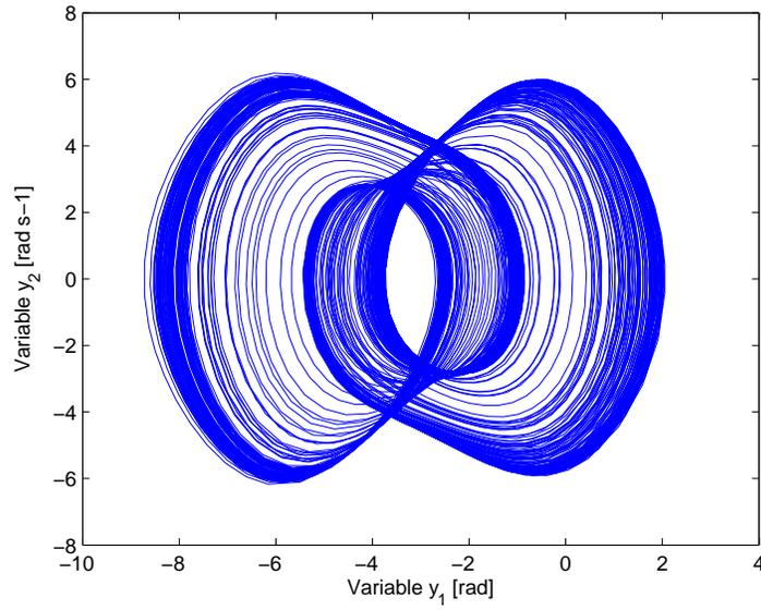
Fig. 3. Chaotic attractor of the non-autonomous horizontal platform system (1) with  $A = 0.3 \text{ kg mm}$ ,  $B = 0.5 \text{ kg mm}$ ,  $C = 0.2 \text{ kg mm}$ ,  $D = 0.4 \text{ kg mms-1}$ ,  $r = 0.11559633 \text{ kg m}$ ,  $R_0 = 6378000 \text{ m}$ ,  $g = 9.8 \text{ ms-2}$ ,  $F = 3.4 \text{ N}$ , and  $\omega = 1.8 \text{ rad ms-1}$ .
