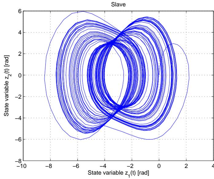
Fig. 11. Simulation result for slave system with the feedback controller gain derived by Proposition 4,  $\tau = 0.24$ , and  $A = 0.3$  kg mm,  $B = 0.5$  kg mm,  $C = 0.2$  kg mm,  $D = 0.4$  kg mms<sup>-1</sup>,  $r = 0.11559633$  kg m,  $R_0 = 6378000$  m,  $g = 9.8$  ms<sup>-2</sup>,  $F = 3.4$  N,  $\omega = 1.8$  rad ms<sup>-1</sup>.
