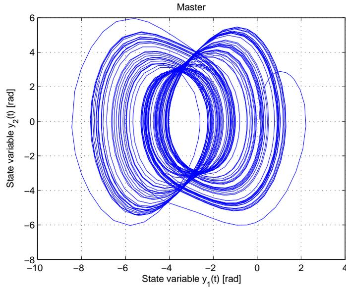
Fig. 10. Simulation result for master system with the feedback controller gain derived by Proposition 4,  $\tau = 0.24$ , and  $A = 0.3$  kg mm,  $B = 0.5$  kg mm,  $C = 0.2$  kg mm,  $D = 0.4$  kg mms<sup>-1</sup>,  $r = 0.11559633$  kg m,  $R_0 = 6378000$  m,  $g = 9.8$  ms<sup>-2</sup>,  $F = 3.4$  N,  $\omega = 1.8$  rad ms<sup>-1</sup>.
