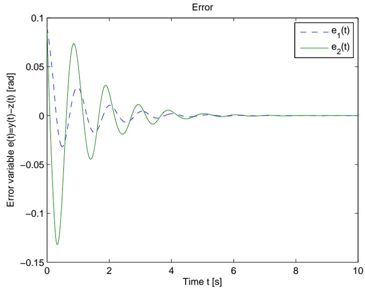
Fig. 6. Simulation result for error system with time delay  $\tau = 0.2318$  and  $A = 0.3$  kg mm,  $B = 0.5$  kg mm,  $C = 0.2$  kg mm,  $D = 0.4$  kg mms-1,  $r = 0.11559633$  kg m,  $R_0 = 6378000$  m,  $g = 9.8$  ms-2,  $F = 3.4$  N,  $\omega = 1.8$  rad ms-1.
