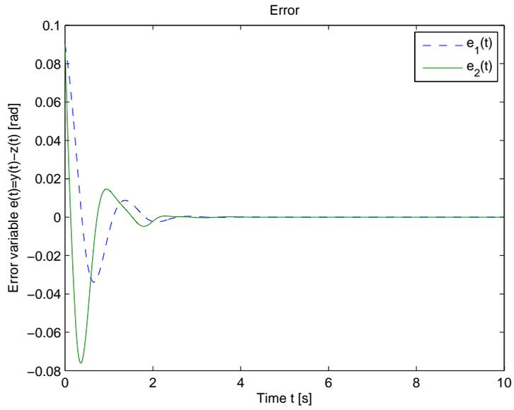
Fig. 12. Simulation result for error system with the feedback controller gain derived by Proposition 4,  $\tau = 0.24$ , and  $A = 0.3 \text{ kg mm}$ ,  $B = 0.5 \text{ kg mm}$ ,  $C = 0.2 \text{ kg mm}$ ,  $D = 0.4 \text{ kg mms-1}$ ,  $r = 0.11559633 \text{ kg m}$ ,  $R_0 = 6378000 \text{ m}$ ,  $g = 9.8 \text{ ms-2}$ ,  $F = 3.4 \text{ N}$ ,  $\omega = 1.8 \text{ rad ms-1}$ .
