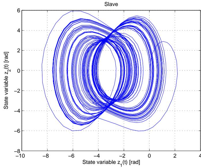
Fig. 8. Simulation result for slave system with the feedback controller gain derived by Proposition 3,  $\tau = 0.24$ , and  $A = 0.3$  kg mm,  $B = 0.5$  kg mm,  $C = 0.2$  kg mm,  $D = 0.4$  kg mms-1,  $r = 0.11559633$  kg m,  $R_0 = 6378000$  m,  $g = 9.8$  ms-2,  $F = 3.4$  N,  $\omega = 1.8$  rad ms-1.
