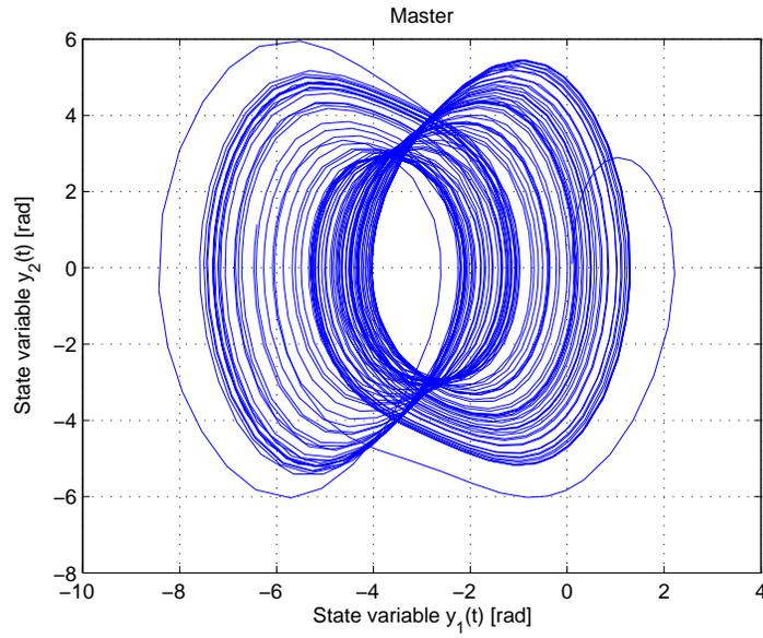
Fig. 4. Simulation result for master system with time delay  $\tau = 0.2318$  and  $A = 0.3 \text{ kg mm}$ ,  $B = 0.5 \text{ kg mm}$ ,  $C = 0.2 \text{ kg mm}$ ,  $D = 0.4 \text{ kg mms-1}$ ,  $r = 0.11559633 \text{ kg m}$ ,  $R_0 = 6378000 \text{ m}$ ,  $g = 9.8 \text{ ms-2}$ ,  $F = 3.4 \text{ N}$ ,  $\omega = 1.8 \text{ rad ms-1}$ .
