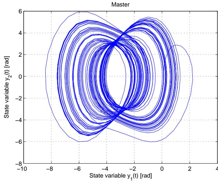
Fig. 7. Simulation result for master system with the feedback controller gain derived by Proposition 3,  $\tau = 0.24$ , and  $A = 0.3 \text{ kg mm}$ ,  $B = 0.5 \text{ kg mm}$ ,  $C = 0.2 \text{ kg mm}$ ,  $D = 0.4 \text{ kg mms-1}$ ,  $r = 0.11559633 \text{ kg m}$ ,  $R_0 = 6378000 \text{ m}$ ,  $g = 9.8 \text{ ms-2}$ ,  $F = 3.4 \text{ N}$ ,  $\omega = 1.8 \text{ rad ms-1}$ .
