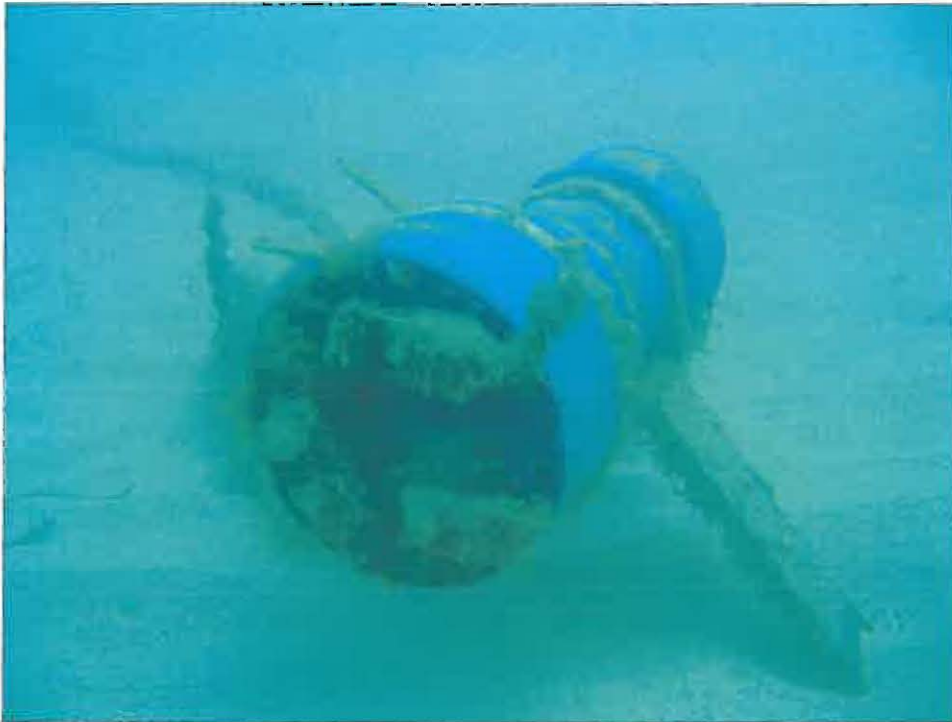
Figure 2. Turbidity logger deployed at Monkey Point.
