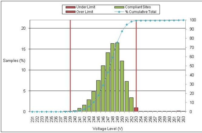
Figure 9. Voltage Distribution of CLVC PQ Meter Sites with ZS AVR and Setpoint
