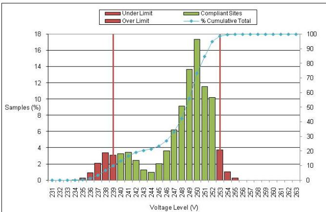
Figure 7. Voltage Distribution of CLVC PQ Meter Sites with Closed Loop Voltage Controller
