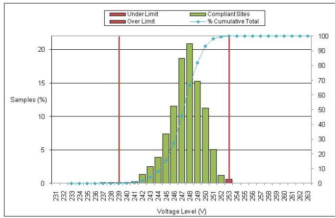
Figure 10. Voltage Distribution of CLVC PQ Meter Sites with Closed Loop Voltage Controller (CVR Mode)
