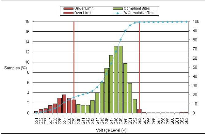
Figure 6. Voltage Distribution of CLVC PQ Meter Sites with ZS AVR and Setpoint
