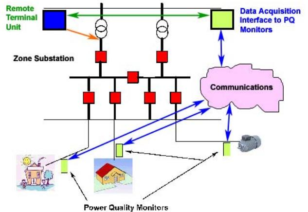
Figure 3. Closed Loop Voltage Control Concept
