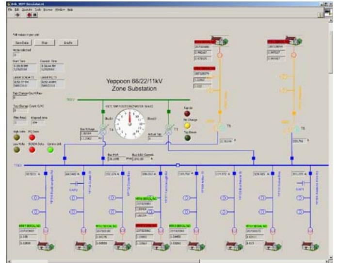
Figure 5. Closed Loop Voltage Control Front Panel
