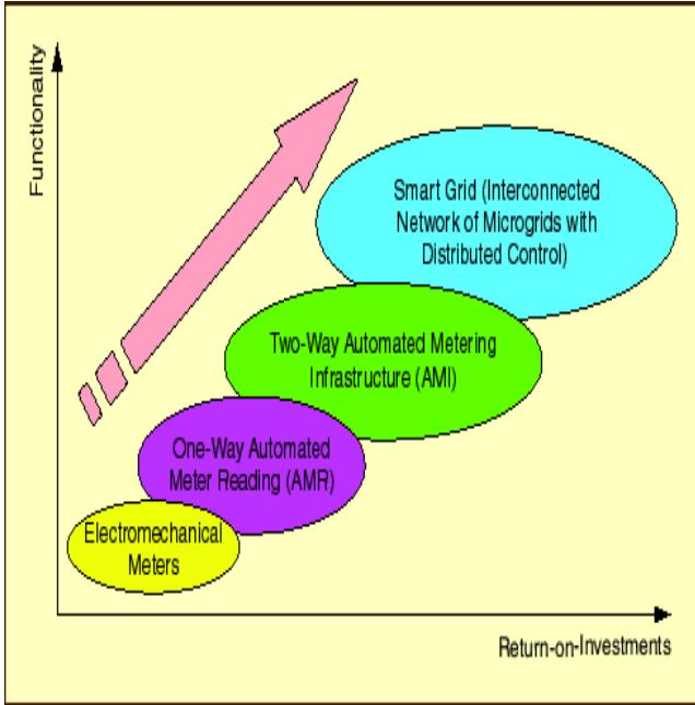
Figure 2: The Evolution of the Smart Grid [2]
