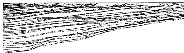
(a) Trajectory of particles (Size 2.5 \mu\text{m} , Injected-50, Collected- 29)
