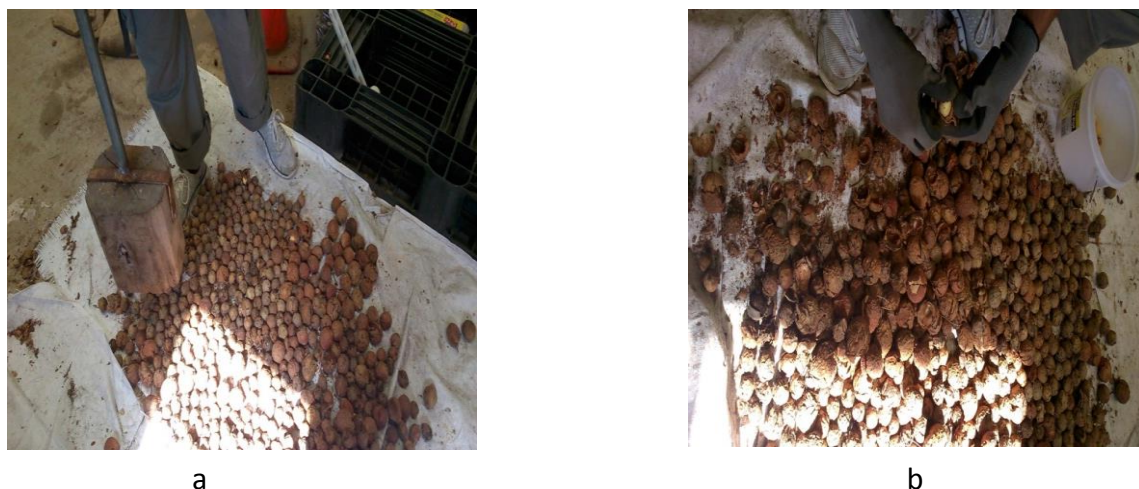
Figure 3.2: (a) BL fruit cracking and (b) kernel separation.
