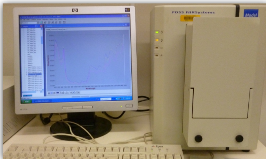
Figure 4.2: Scanning grating instrumentation (NIRS Systems 6500, FOSS).
