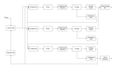
Fig. 1. A simplified model of the pan stage showing process material flows and equipment interactions.
