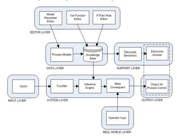
Fig. 2. Smart supervisory control system framework diagram.
