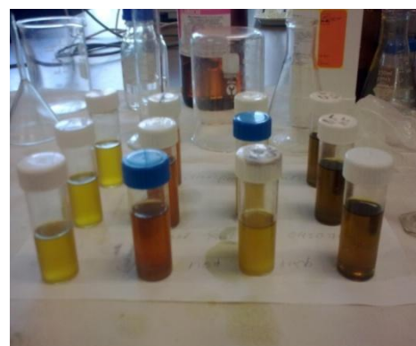
Fig. 7. FAME derived from different methods (from left; base catalysed, acid catalysed, 3-stage, 4-stage).
