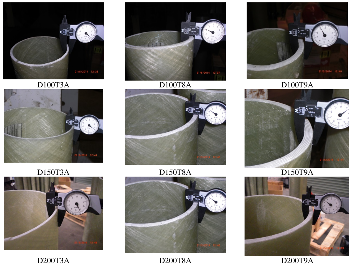
Figure 7: FRP tubes with a variety of diameters and wall thicknesses
