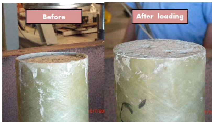
Figure 40: De-bonding between FRP tube and concrete column
