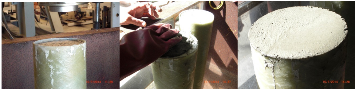
Figure 15: Filling the gaps with mortar
