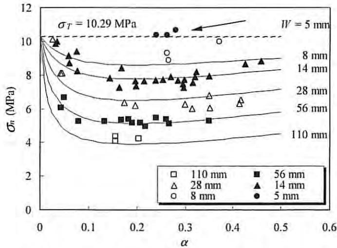
Figure 2. Comparisons of experimental results [10] with predictions from the boundary effect model.
