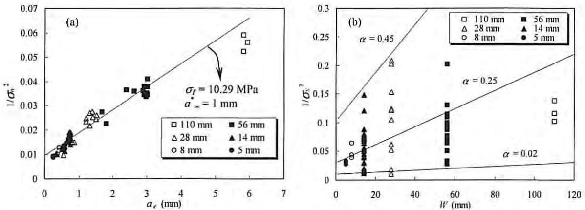
Figure 3. (a) Determination of material constants  $\sigma_T$  and  $a_m^*$ , and (b) predictions from the from the boundary effect model.
