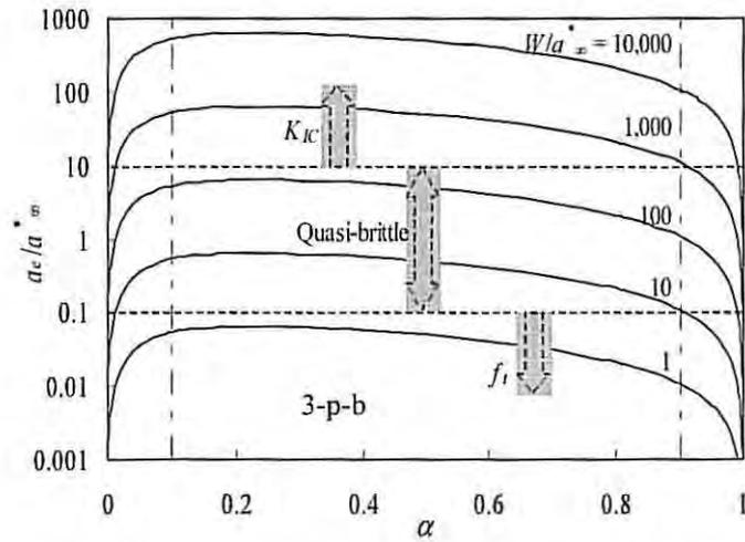
Figure 4. Fracture transition zones of 3-p-b specimens showing the influence of specimen size and boundaries.
