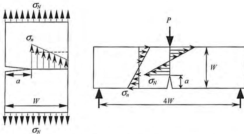
Figure 1. Single edge notched tension (SENT) and 3-point-bending (3-p-b) specimens with two nominal strengths:  $\sigma_N$  does not consider the presence of the crack,  $\sigma_n$  considers the crack.
