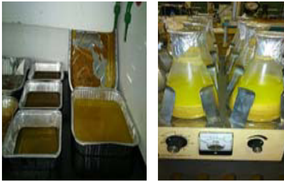
Fig. 4. Chemical oil extraction (left side: oil yield in the trays and right side: conical flasks with oil content in the shaker machine)
