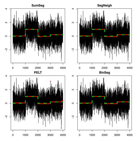
Figure 1: Recovery of known level changes (green) from the four algorithms on simulated data (in red): **SumSeg, SegNeigh, BinSeg** and **PELT**. The simulated data has length N=4000, level changes at 1000, 2000, and 3000, and the means for each segment are 0, 1, 0, and 0.2 with introduced random noise mean=0 and SD=1. The PELT algorithm introduced a number of small additional breaks (false positives). The computation time was SumSeg=0.054s SegNeigh=37.272s PELT=0.231s BinSeg=0.338s.
