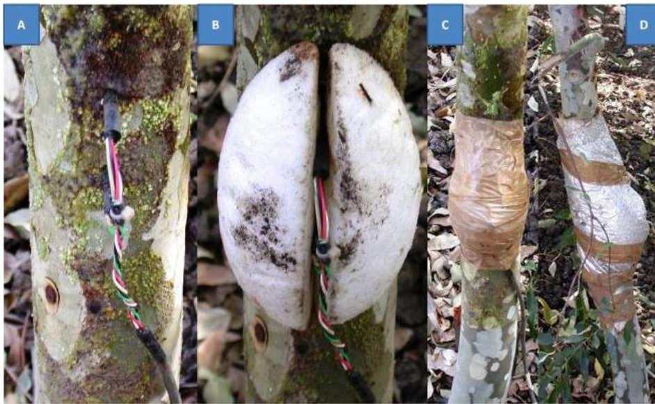
Figure 5.1: Installation of a TDP sensor
