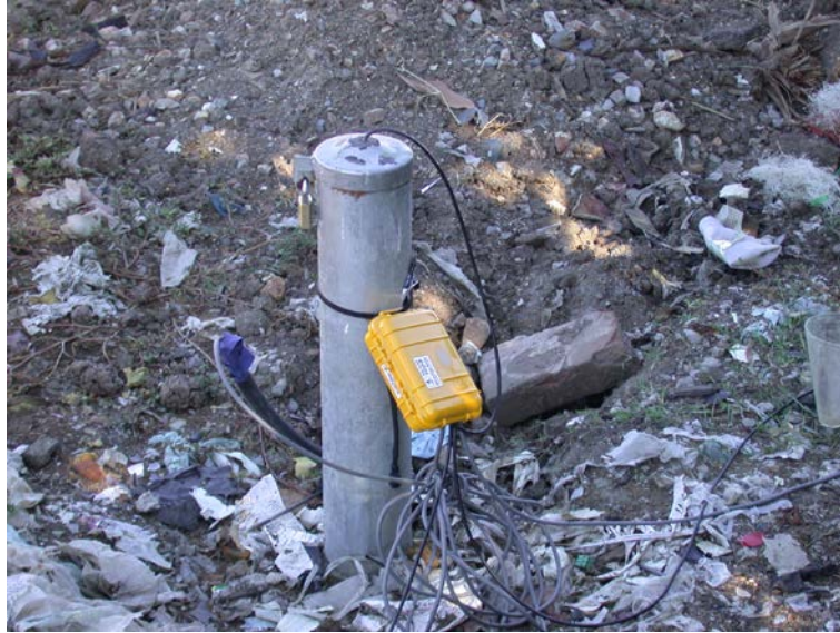
Figure 2.18: Piezometer tube completely protected with metal casing
