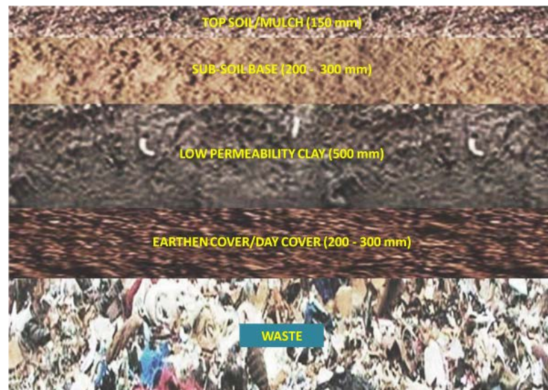
Figure 1.2: Typical clay capping system in Queensland Source: (EPA 2005)
