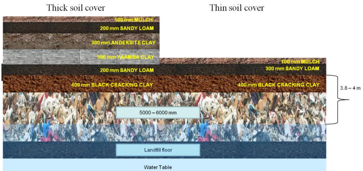
Figure 2.8: Different types of soils and their depths used in Thick (left) and Thin (right) phytocaps
