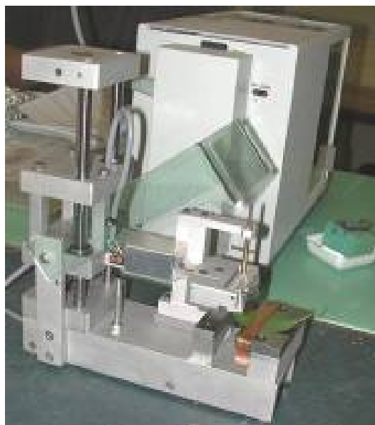
Figure 6.4: Leaf toughness tester
