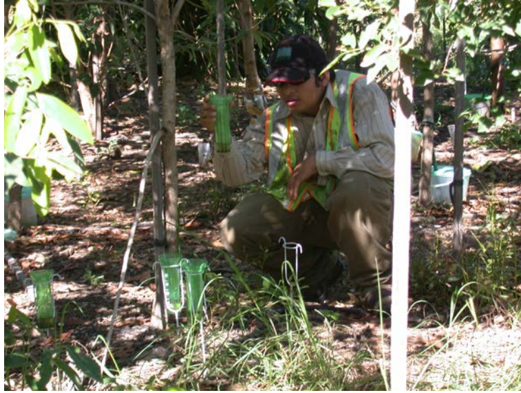
Figure 6.3: Standard rain gauge used in measuring throughfall
