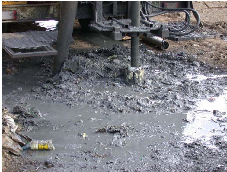
Figure 2.17: Wet waste samples from 6 m depth
