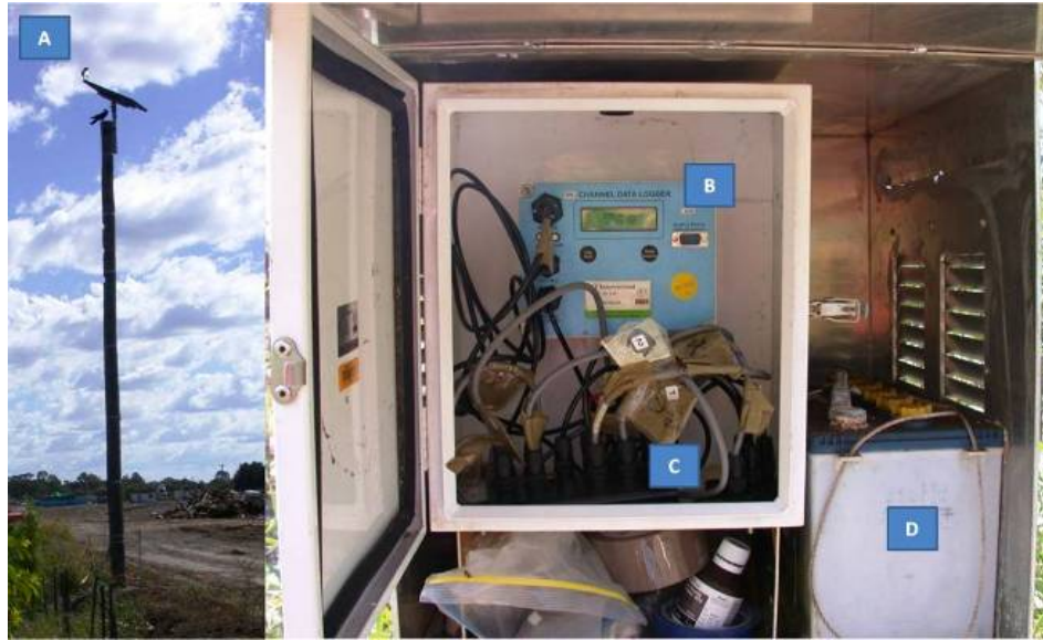
Figure 5.2: Power and sensor system used to measure sapflow A) solar panel, B) smart logger, C) monibus bar and D) battery
