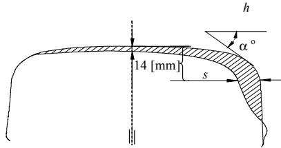
Fig 3. Central vertical wear  $h$  and side wear  $s$
