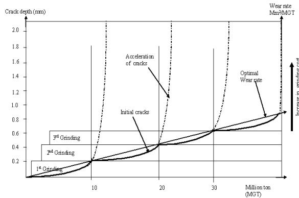
Fig 2. Achieve balanced wear by reducing cracks [14]
