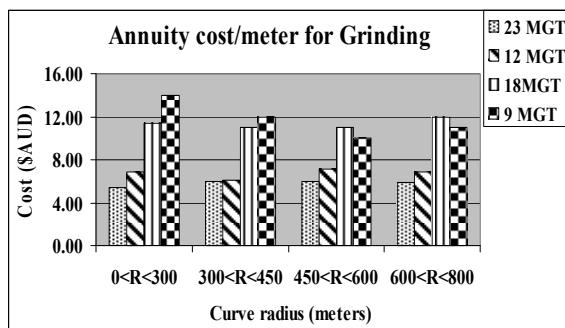
Fig 6. Annuity cost/m for grinding 0 to 800 m curves
