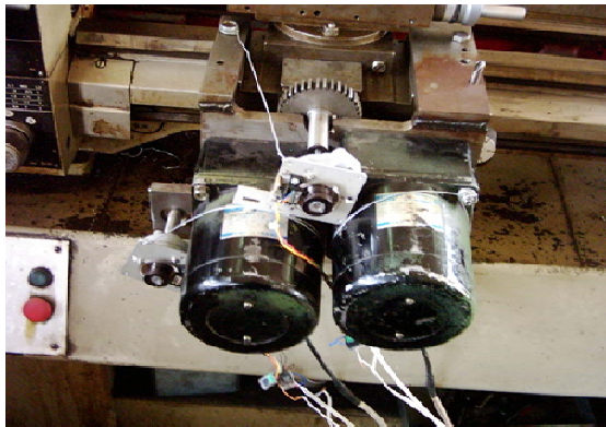
Figure 5. Encoder assemblies with the adapter plate of the feedback control system.
