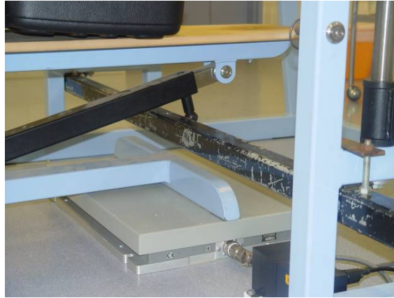
Figure A.7. Custom made force plate mounted bench press.
