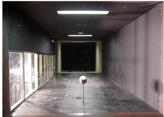
Fig. 2: Experimental set up in RMIT Industrial Wind tunnel with a Rugby ball
