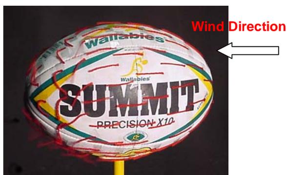
Fig. 4: Flow structure around a rugby ball at 0° yaw angle
