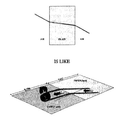
Figure 3: A pair of wheels rolling form a hard to a soft surface change direction like a ray of light passing from air into glass.
