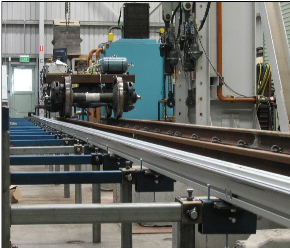
Figure 6.27. Instrumented Bogie with DAQ ready for commissioning
