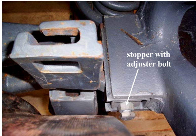
Figure 6.11. Brake beam stopper of the non-braked wheelset
