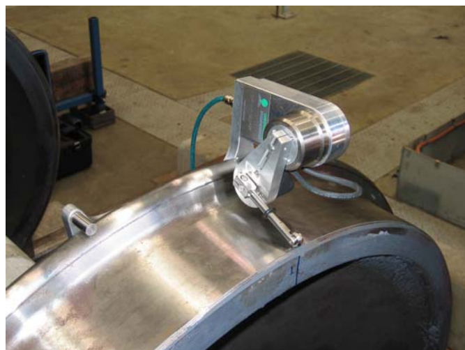
Figure 6.19. MiniProf tool for measuring the wheel profile
