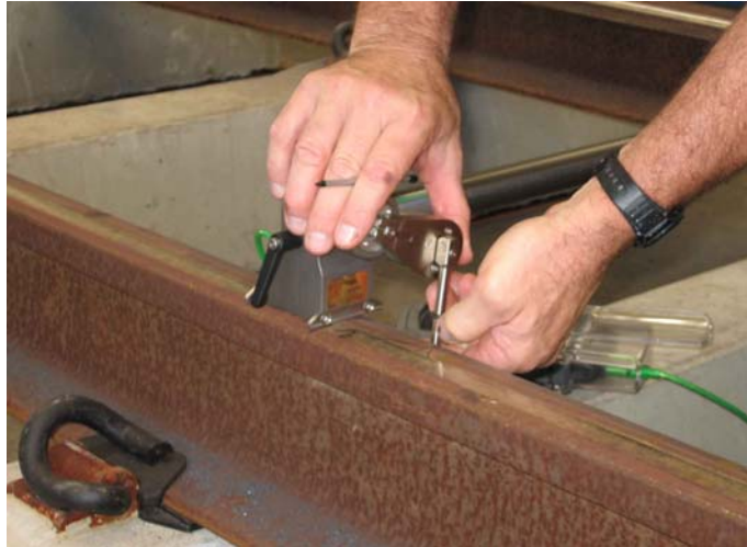
Figure 6.20. Measurement of the rail profile using MiniProf
