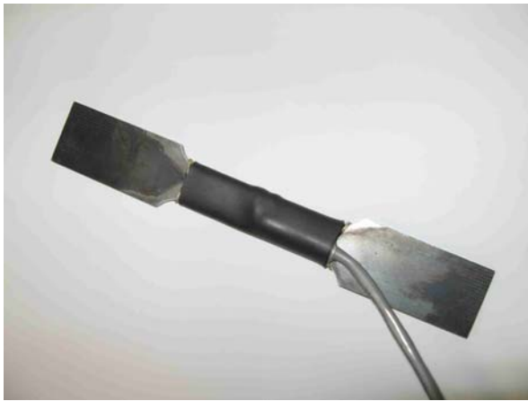
(a) part of the hanger with strain gauge
