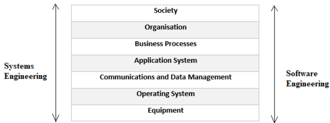
Figure 2. 2 The layers of an information system.
