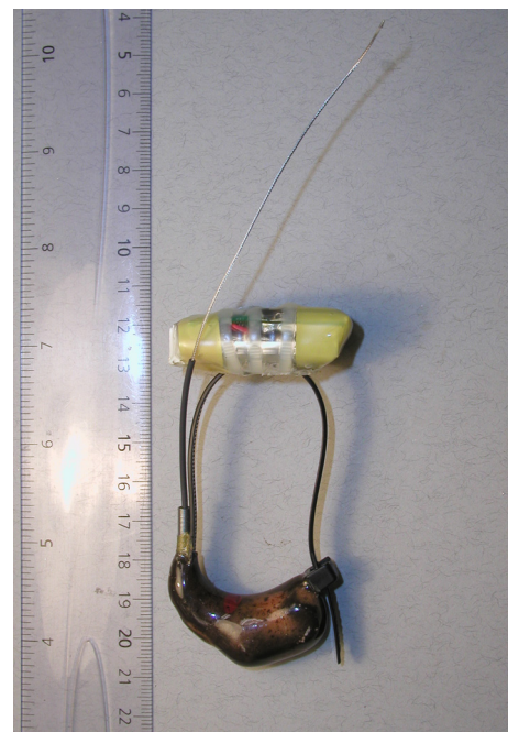
Figure 2. Complete GPS radio collar ready for fitting.
