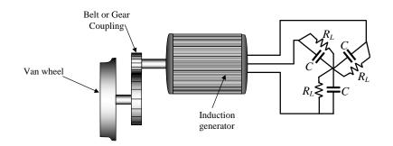
Figure 1 Electrical braking system using an induction generator (adapted from [2])
