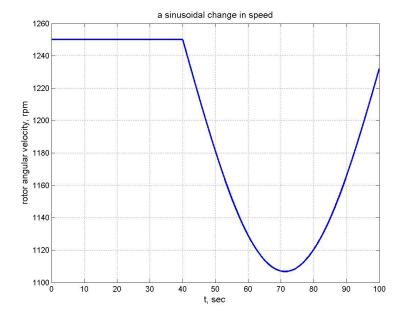
Figure 4 A change in the machine shaft speed occurring at t = 40 sec
