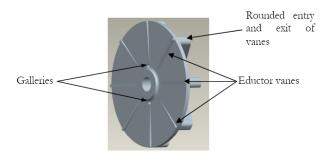
Figure 9: Features of Impeller
