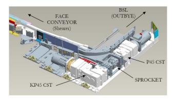
Figure 2: Typical maingate using two(2) CST Gearboxes
