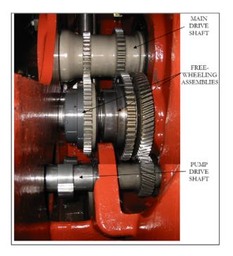
Figure 6: Cooling pump drive-train 45 CST
