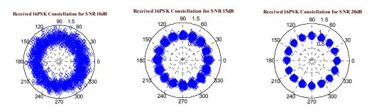
Figure 7. Received 16PSK constellation for corresponding SNR values of 10dB, 15dB and 20dB
