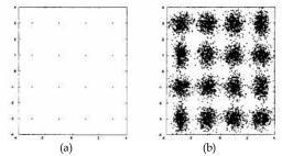
**Figure 2.** Phase noise effects on 16-QAM modulated OFDM signals (a) original 16-QAM constellations (b) 16-QAM constellations corrupted by phase noise
