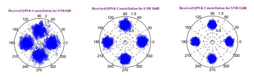
Figure 6. Received QPSK constellation for corresponding SNR values of 6dB, 10dB and 12dB
