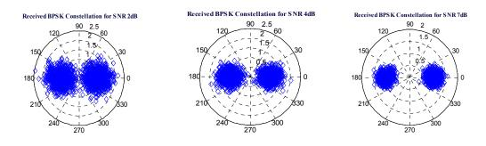
Figure 5. Received BPSK constellation for corresponding SNR values of 2dB, 4dB and 7dB
