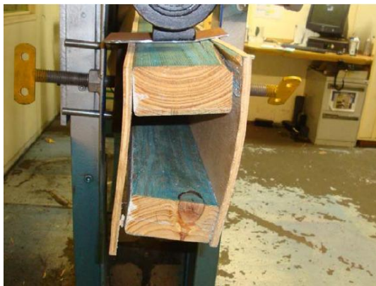
Fig 5. Beam #1 failed along both glue lines
