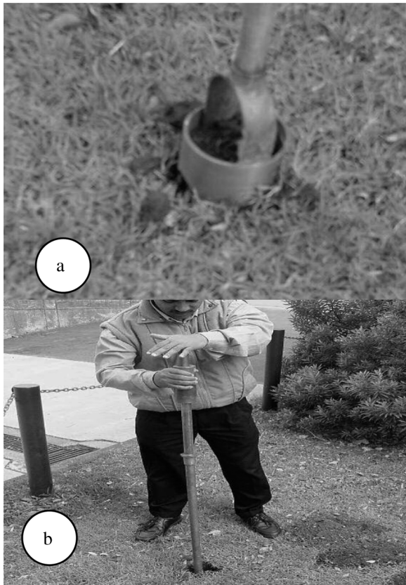
Fig. 2. Procedures for sample collection and measuring the depth of drill. (a). Drilling with the auger. (b) Sample extraction.
