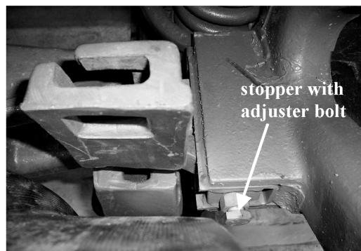
Figure 6 Brake beam stopper of the non-braked wheelset
