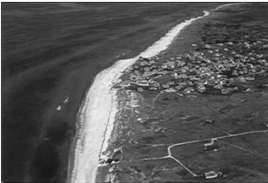
Figure 18. Aerial photo of the same location in 1999, 15 months after the implementation of pressure equalisation modules. ( www.skagen-innovation.dk )
