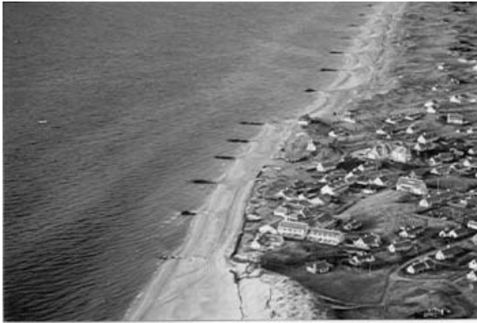
Figure 17. Aerial photo of the groynes at Gl. Skagen, before the implementation of pressure equalisation modules. ( www.skagen-innovation.dk )
