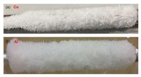
Figure 8.11: Crystallisation scale deposition on pipe surface (a) Cu and (b) Al, concentration of 4.50 mol/dm<sup>3</sup>, bulk temperature 48°C, surface temperature - $3.6^{\circ}$ C, coolant temperature - $4^{\circ}$ C and exposure time 170 minute
