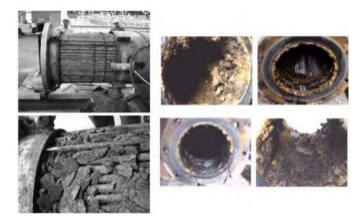
Figure 2.10: Negative effect of excessive inlet baffle spacing on deposit formation (left, (Müller-Steinhagen, 2011)) and scale growth observed in components of the pipe (right, (Nawrath et al., 2006))
