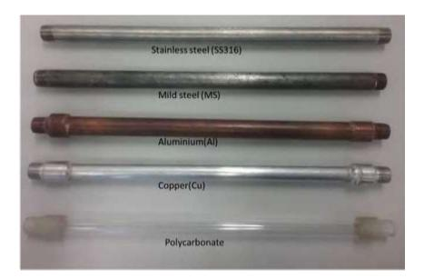
Figure 8.3: Experimental test pipes with different materials
