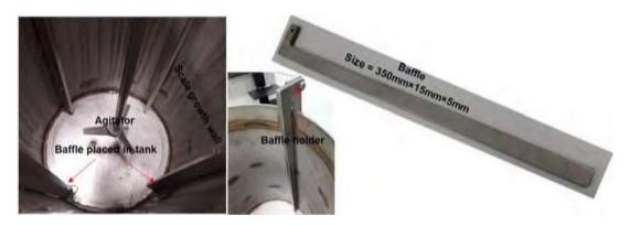
Figure 4.7: Position of baffle and agitator in the tank
