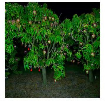
Figure 6. A tracking example: red bounding boxes indicate tracked fruit with valid assignments; pink indicates predicted location for fruit on the track list that were not detected in the current frame; blue indicates a new fruit detection. Numbering on fruit is in order of detection. Red arrows point to fruit mentioned in text.
