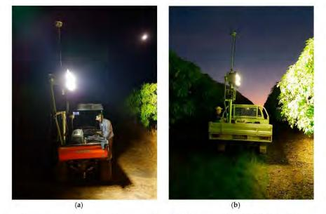
**Figure 1.** Automated imaging platform, involving a GNSS device (on pole), a 720 W LED floodlight, and a camera, powered by an inverter-generator and mounted on a farm vehicle ((**a**) buggy or (**b**) utility), operated at 5 km/h.
