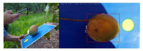
Figure 4. In-field imaging (left) and the result of fruit sizing mobile app (right)
