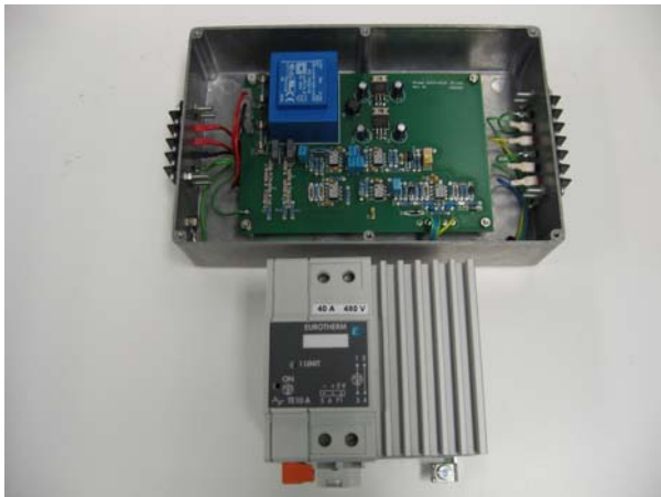
Fig15. Voltage Control System and Commercial 480Vac, 40Arms Thyristor Phase Controller.
