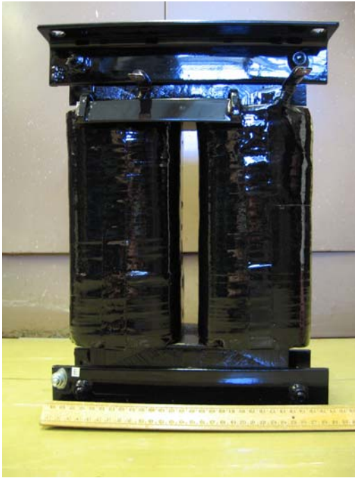
Fig 14. Voltage Control Reactor –12.5 kVA, 480Vrms.
